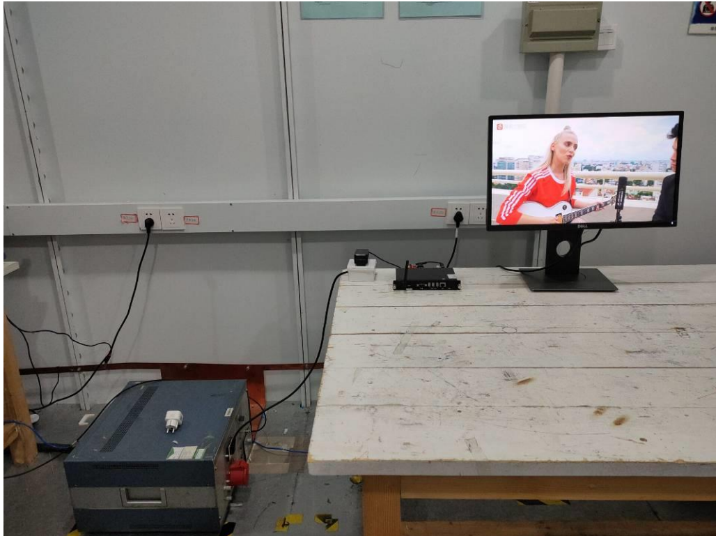
Photo of Conducted Emissions Measurement
