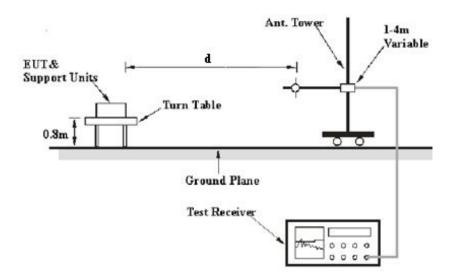
The radiated emission tests were performed at the 3 meters distance, above 1GHz were performed at the 3 meters, using the setup accordance with the ANSI C63.4-2014. The specification used was the FCC Part 15.109 Class B limits.
