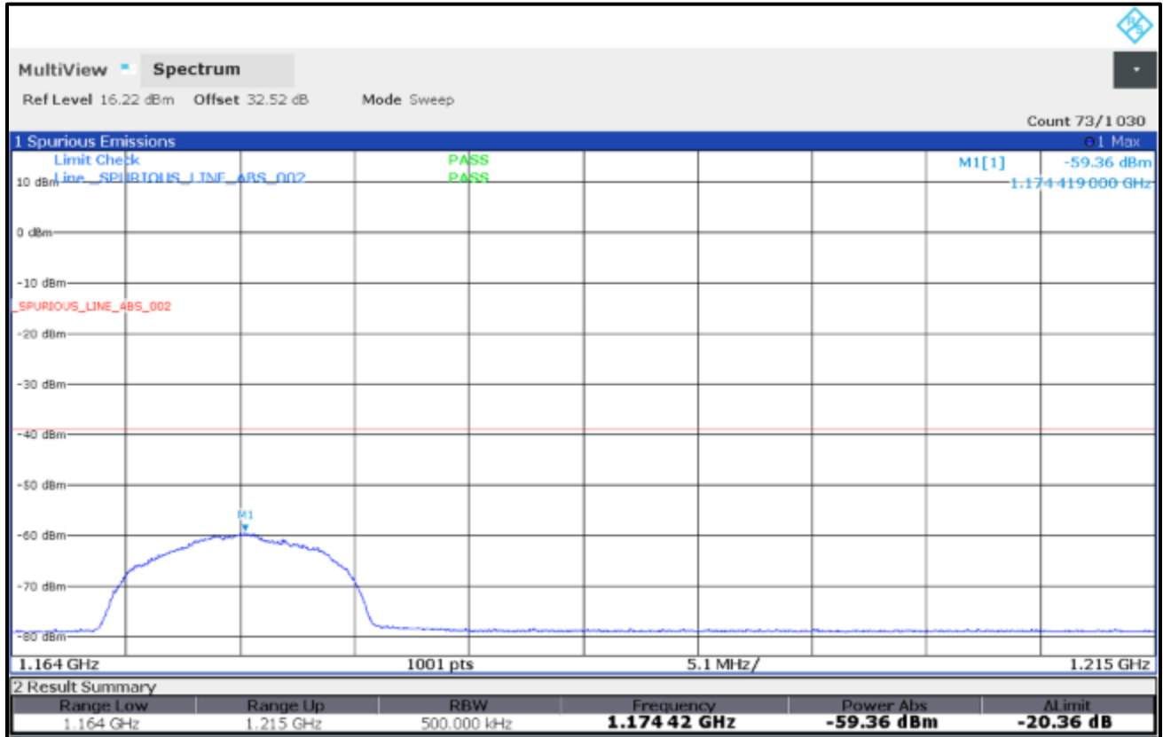
Plot 7-11: Radio Navigation Satellite Services Emissions – 587.0 MHz (1174.419 MHz); 1164-1215 Band
