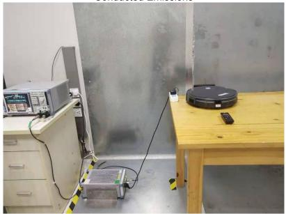
Radiated Spurious Emissions From 30MHz-1000MHz
