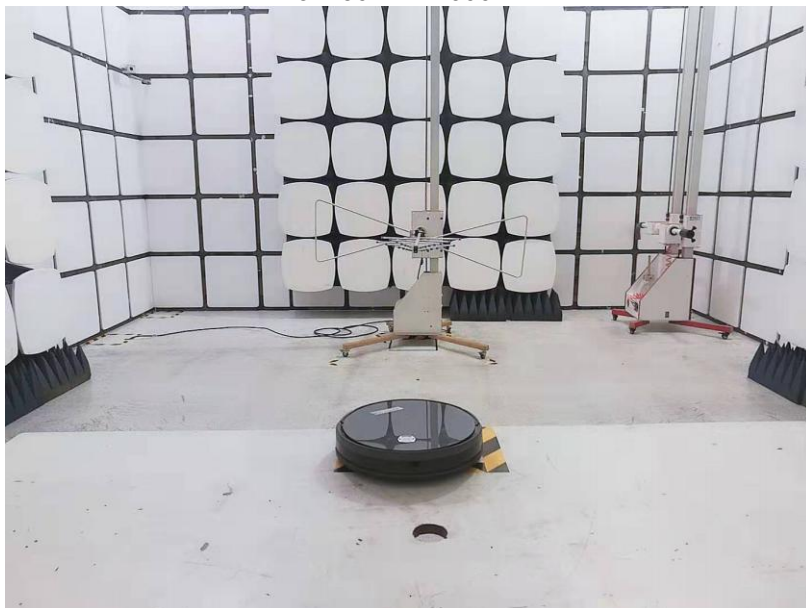
Radiated Spurious Emissions From 30MHz-1000MHz
