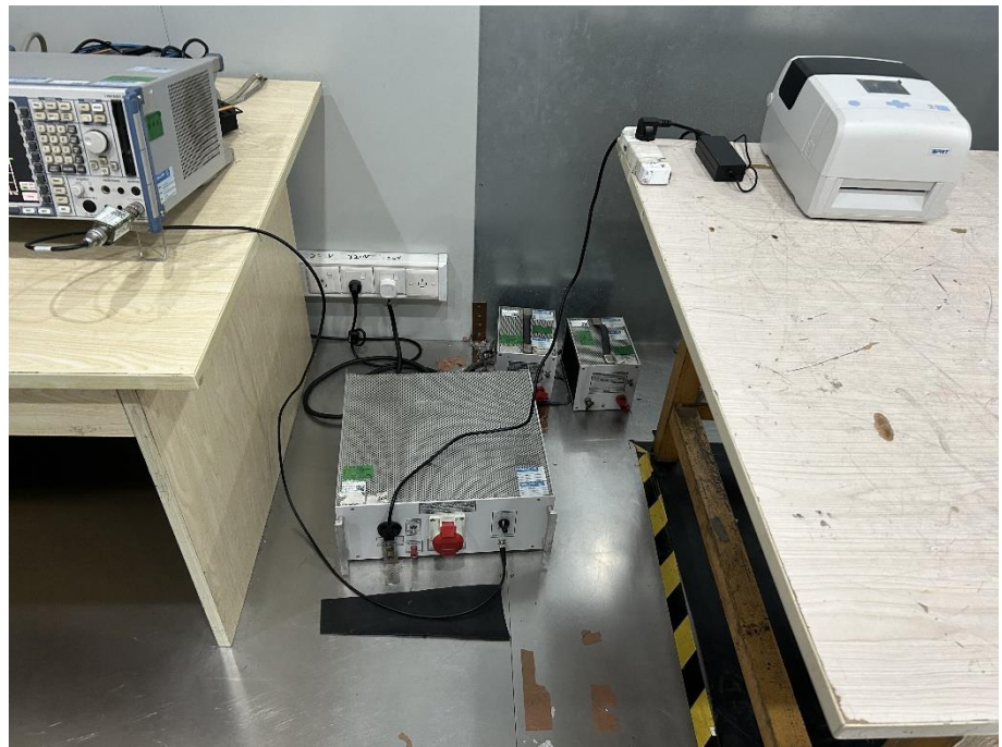
Conducted Emission Test Setup
