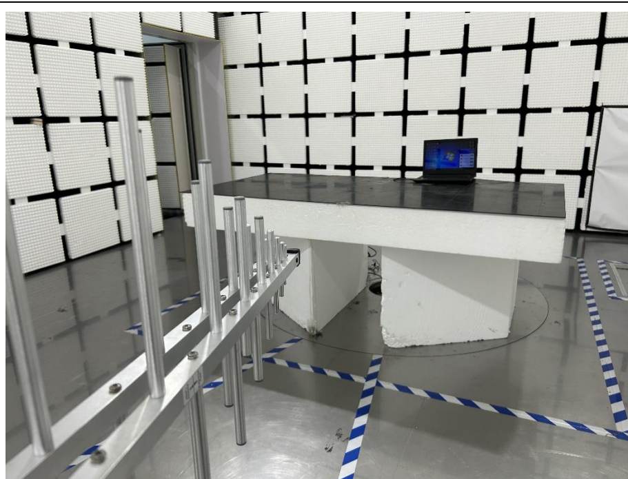
Radiation Emission Test Setup (30MHz to 1GHz)
