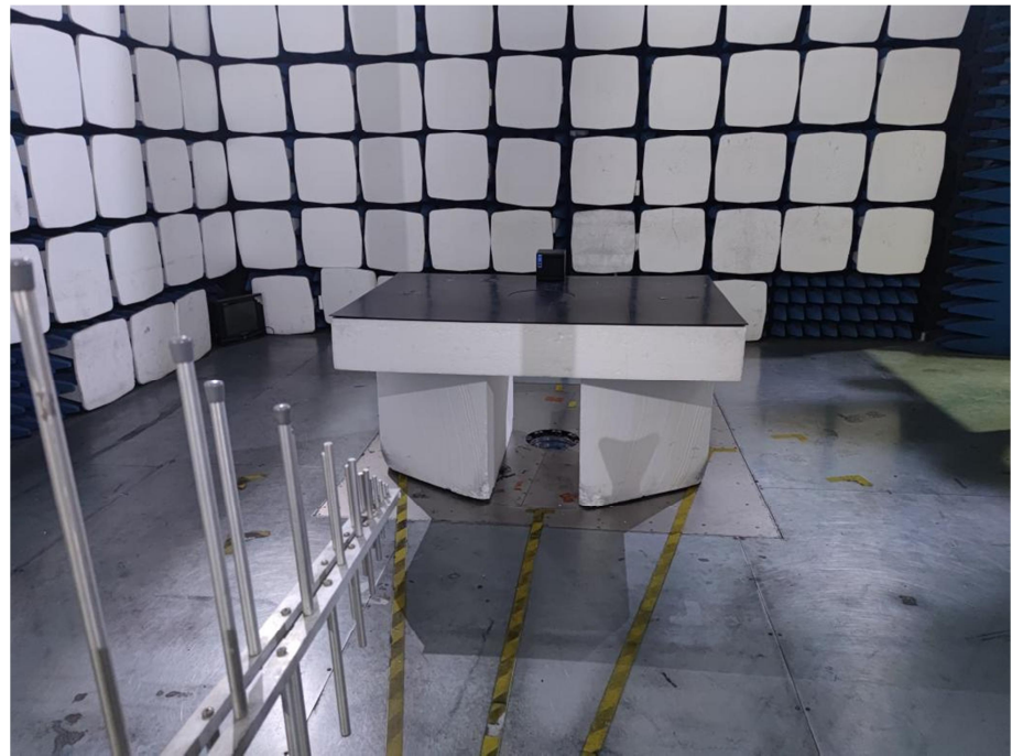
Radiation Emission Test Setup (30MHz to 1GHz)
