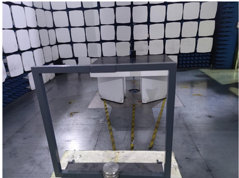
Radiation Emission Test Setup (Below 30MHz)
