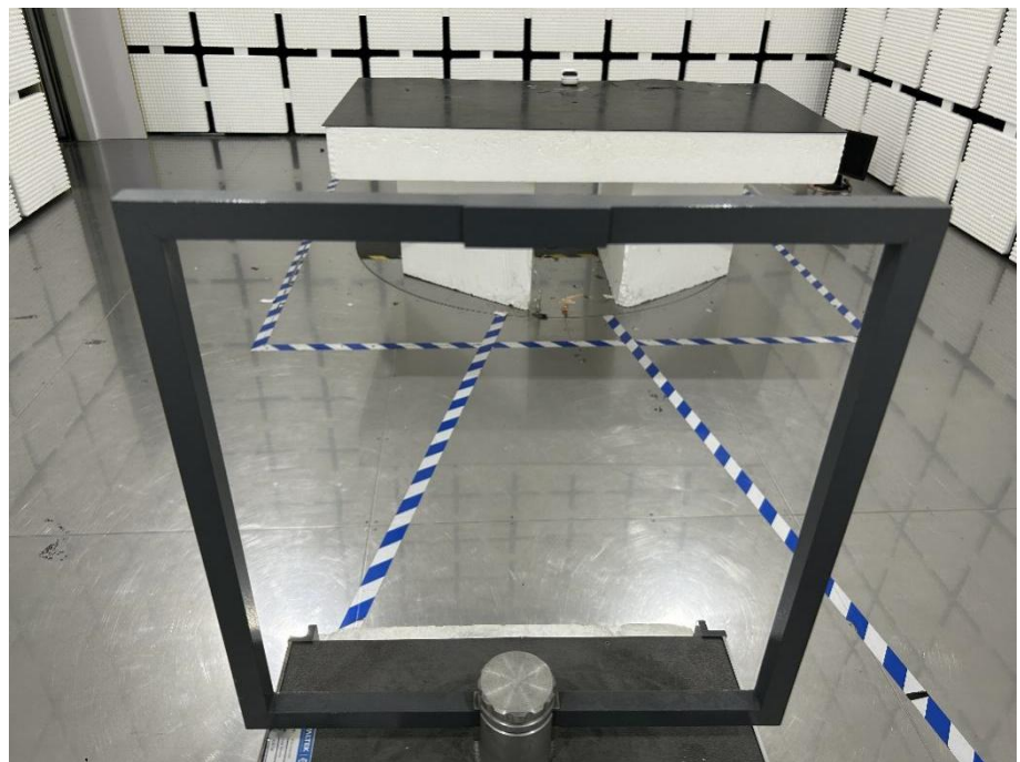
Radiation Emission Test Setup (Below 30MHz)
