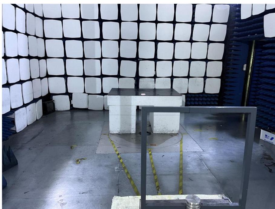
Radiation Emission Test Setup (Below 30MHz)
