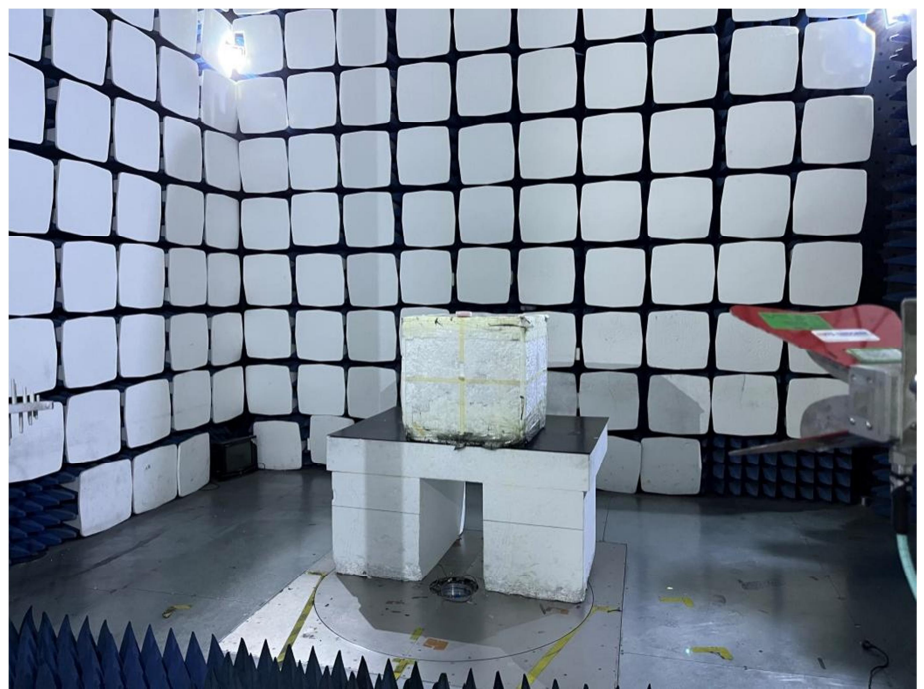
Radiation Emission Test Setup (1GHz to 18GHz)
