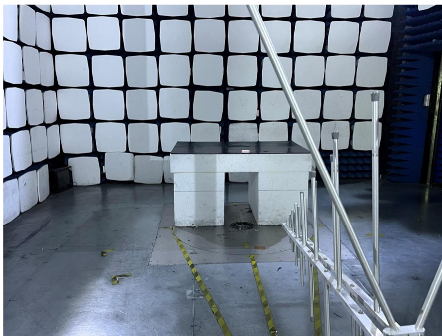
Radiation Emission Test Setup (30MHz to 1GHz)
