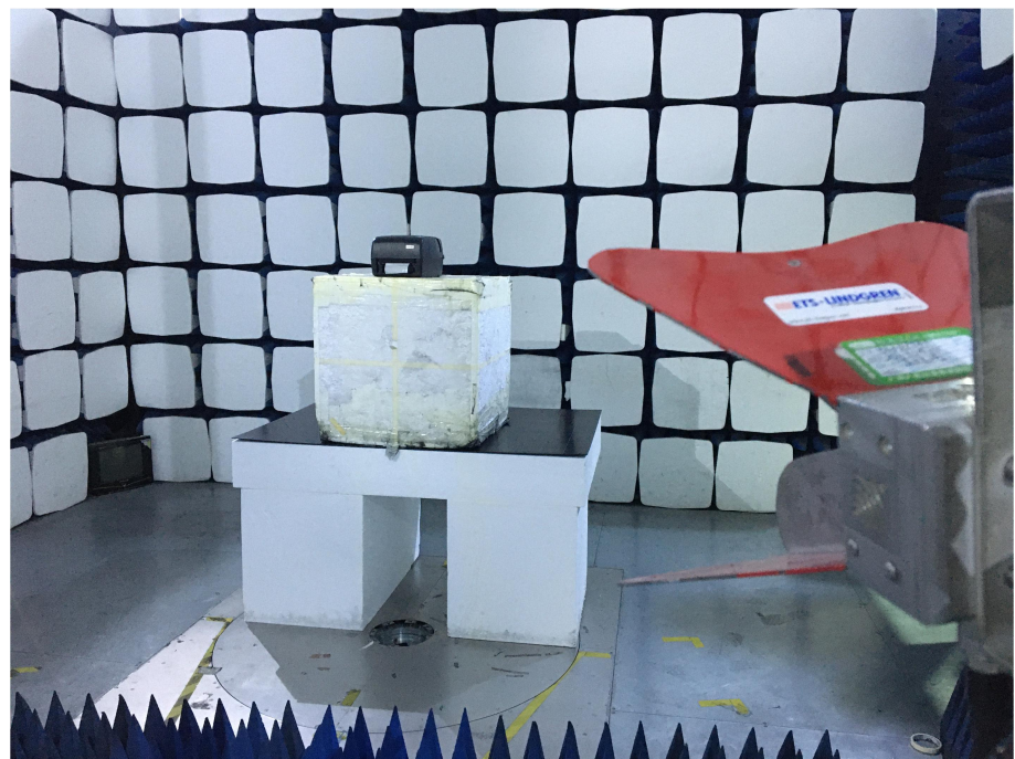
Radiation Emission Test Setup (1GHz to 18GHz)
