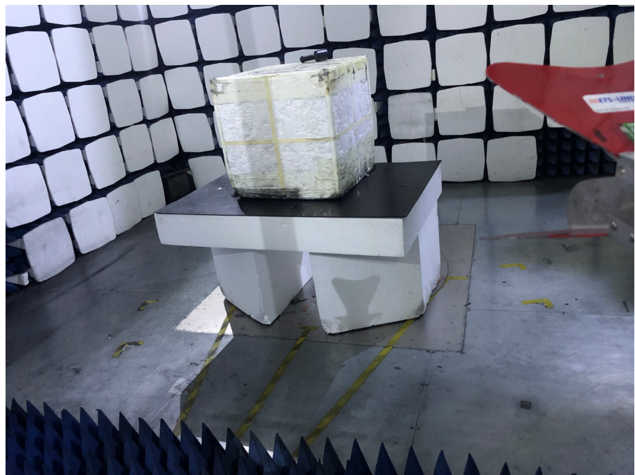
Radiation Emission Test Setup (1GHz to 18GHz)
