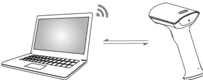
The scanner is powered on by pressing the scanning button, and connect it to the host devices through Bluetooth. The green light indicates that it is connected and can be used normally.
