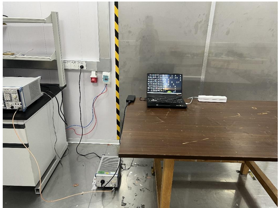
Conducted Emission Test Setup
