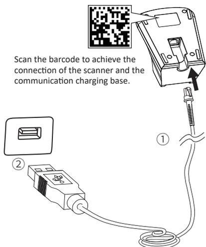
Scan the barcode to achieve the connection of the scanner and the communication charging base.
