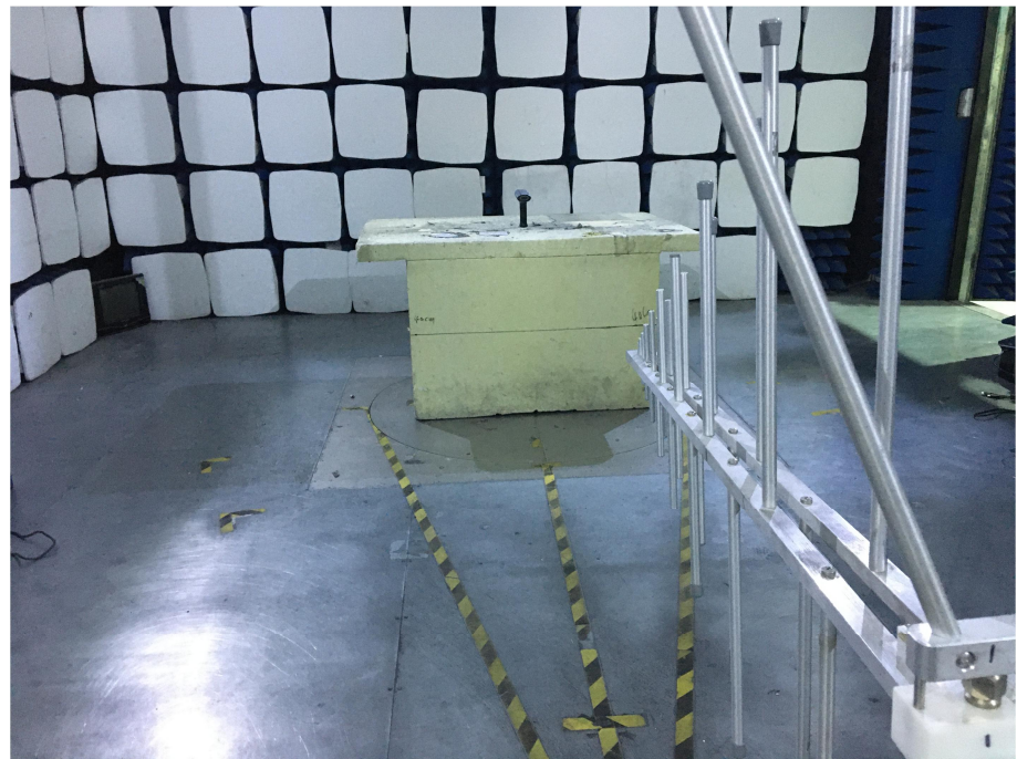
Radiation Emission Test Setup (30MHz to 1GHz)
