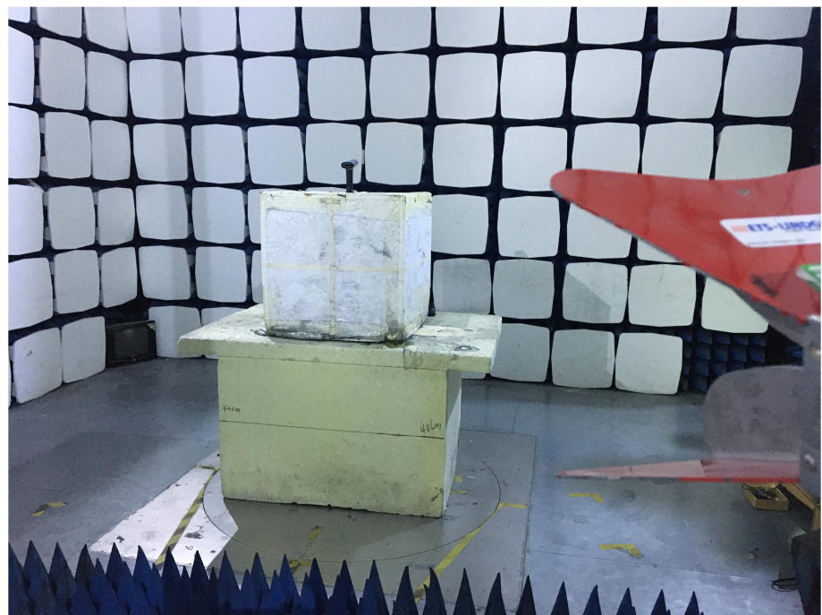
Radiation Emission Test Setup (1GHz to 18GHz)
