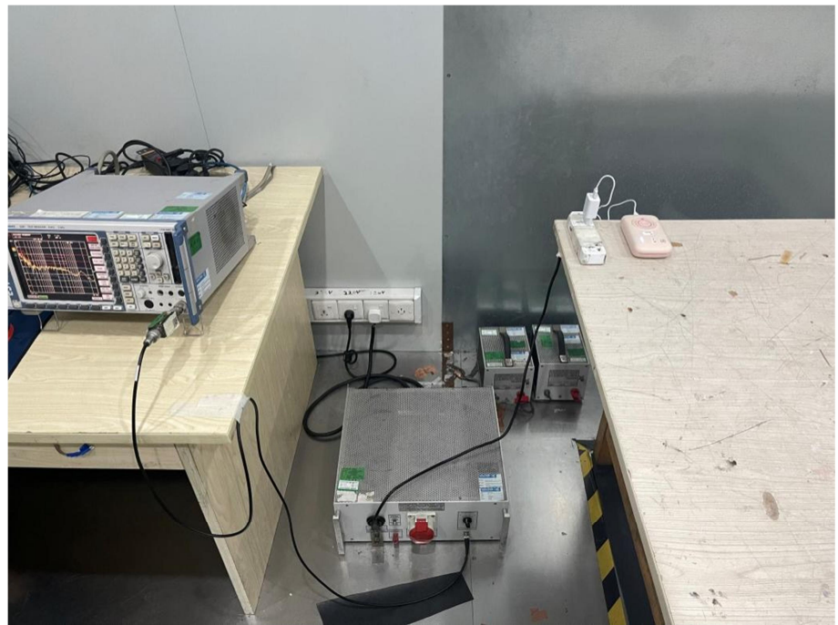
Conducted Emission Test Setup
