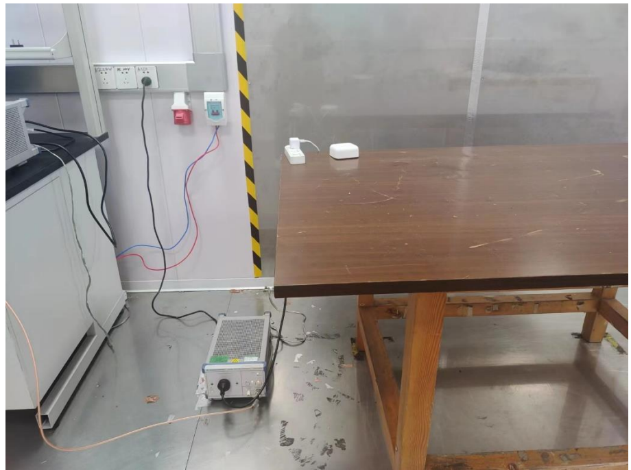
Conducted Emission Test Setup
