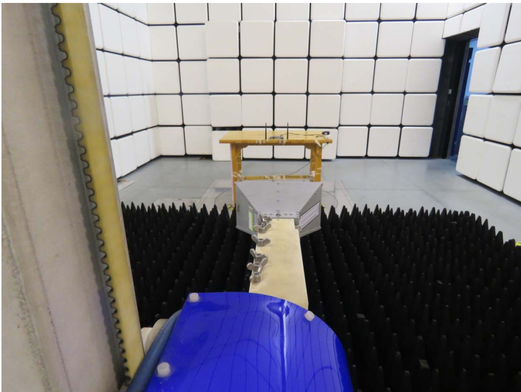
Picture 2: Radiated Spurious Emissions Test setup
