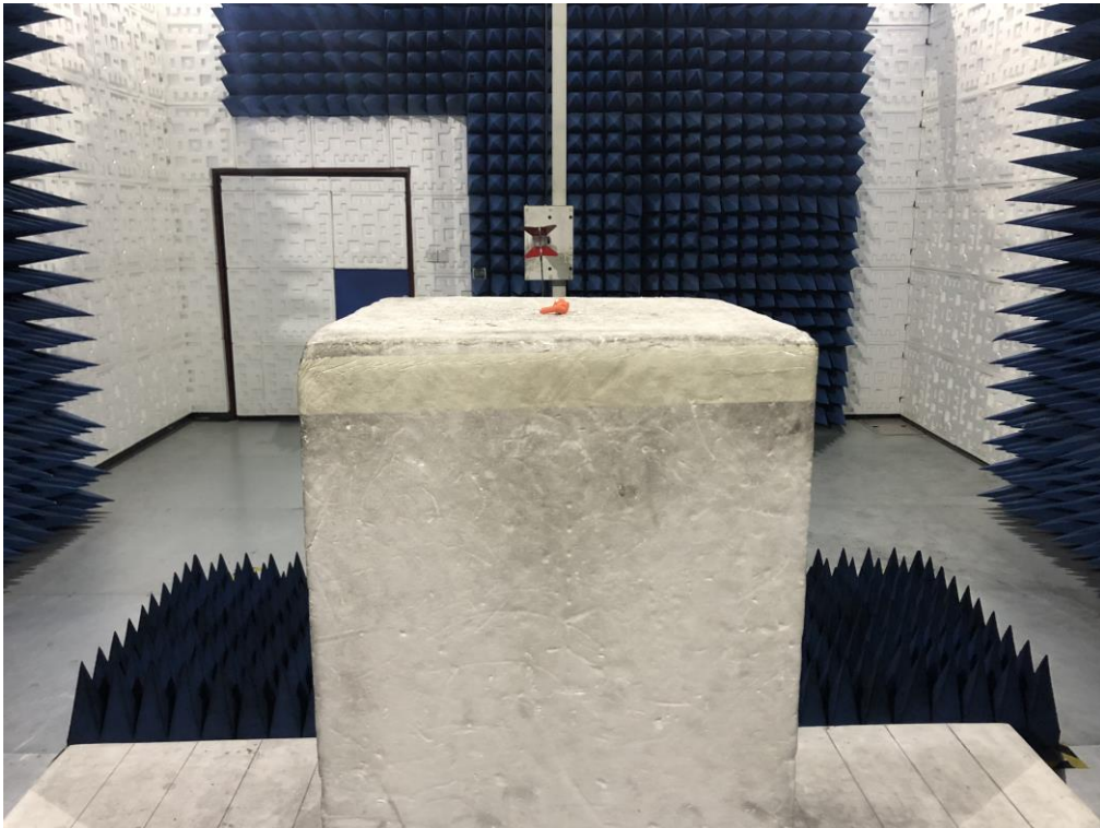
RADIATED EMISSION TEST SETUP ABOVE 1GHZ
