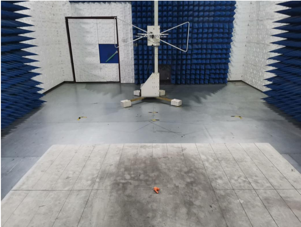
RADIATED EMISSION TEST SETUP ABOVE 1GHZ
