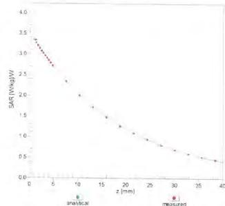
$f = 1900 \text{ MHz}, \text{WGLS R22 (H\_convF)}$
