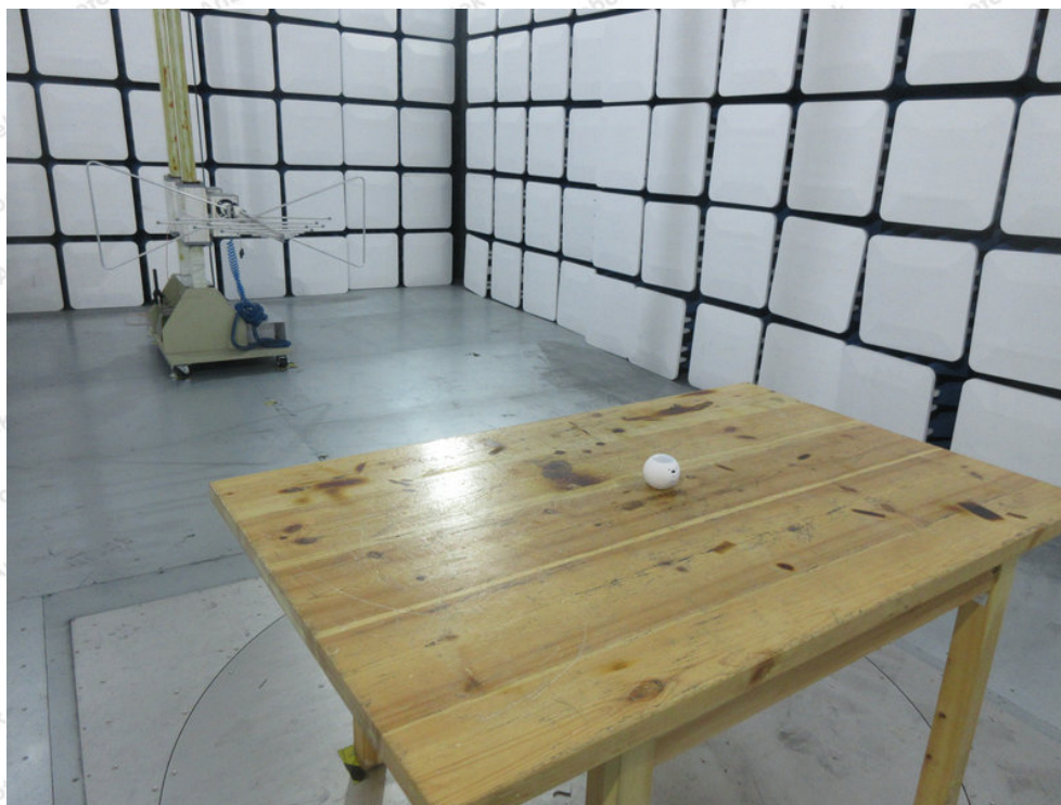
Photo of Radiation Emission Test
