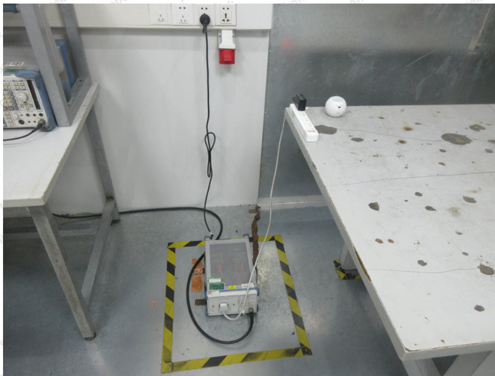
Photo of Conducted Emission Measurement
