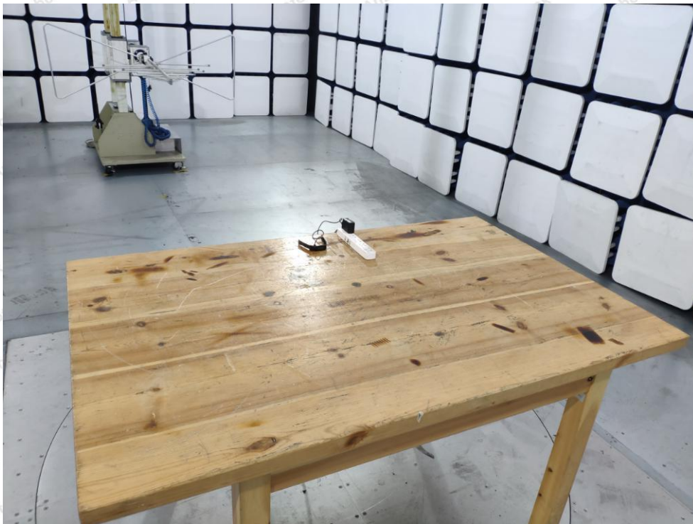
Photo of Radiation Emission Test
