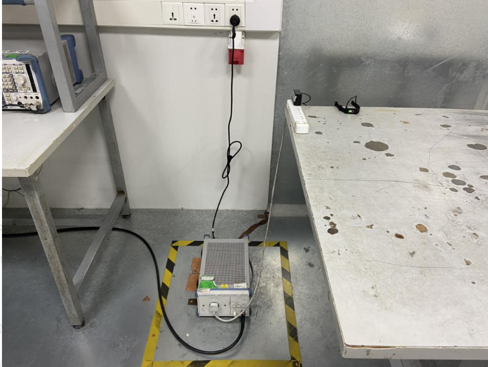
Photo of Conducted Emission Measurement
