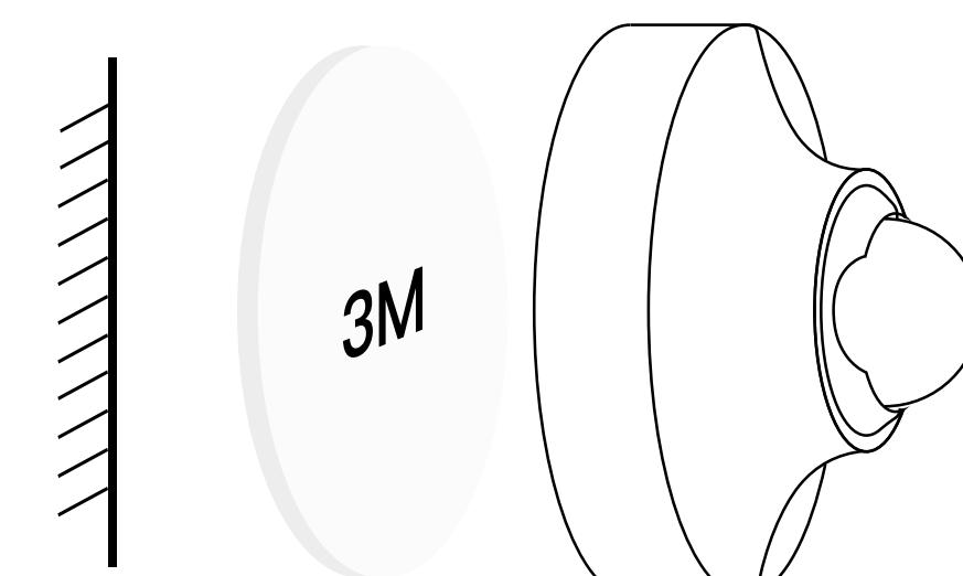
Tighten the camera, and clamp the snap. Adjusts the camera angle according to the display of the mobile phone
