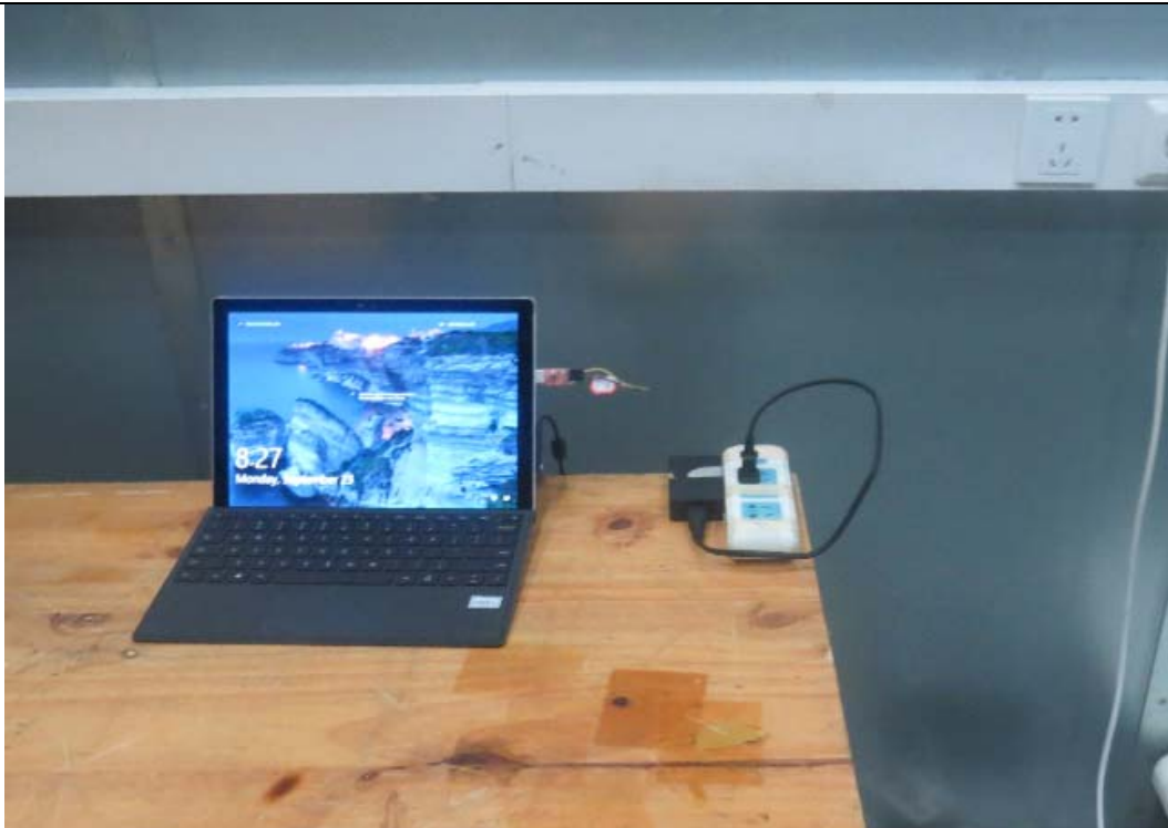
Picture 2 Conducted Emission Test Setup
