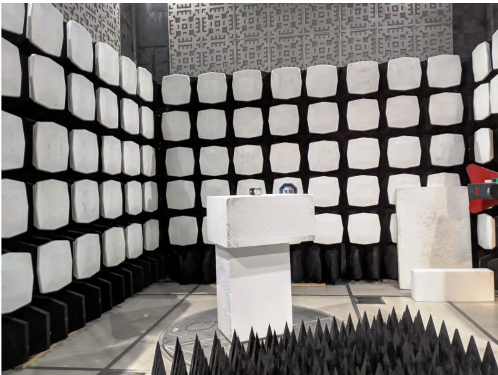
Figure 6: Equipment Under Test – Radiated Emissions >1GHz
