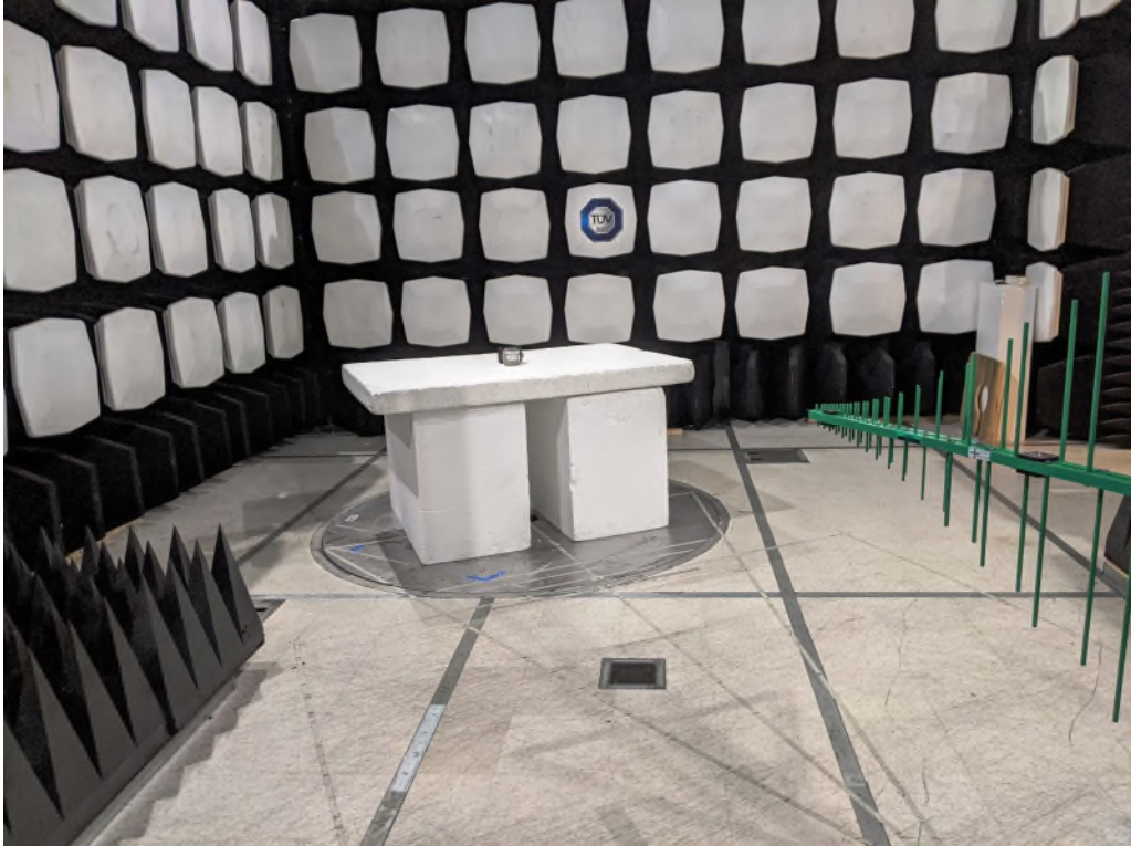
Figure 4: Equipment Under Test – Radiated Emissions <1GHz
