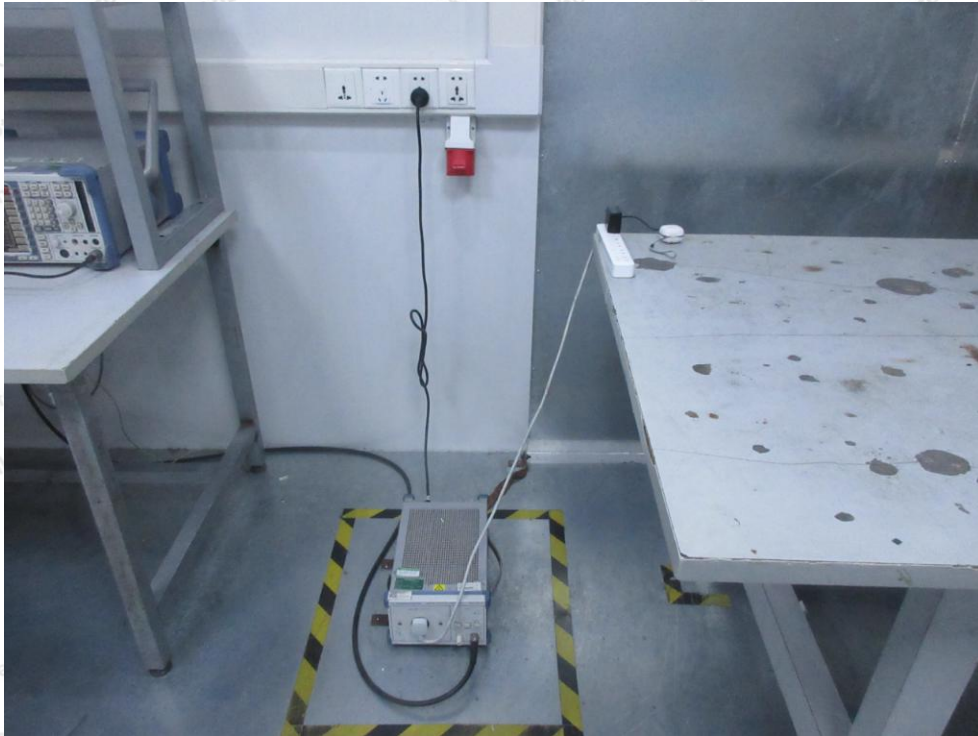
Photo of Conducted Emission Measurement
