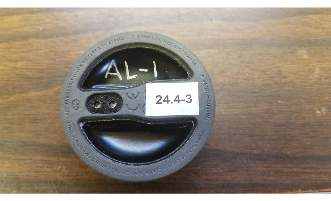
Top View of the Aluminum Enclosure - This is the top part of the EUT and was taken to show the difference between this and the plastic enclosure.
