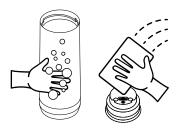
ALWAYS STORE BOTTLE WITH THE LID & SENSOR PUCK REMOVED to allow parts to dry completely.
