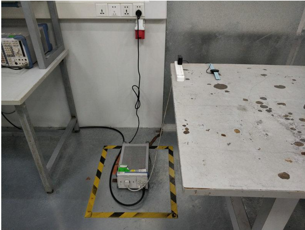
Photo of Conducted Emission Measurement
