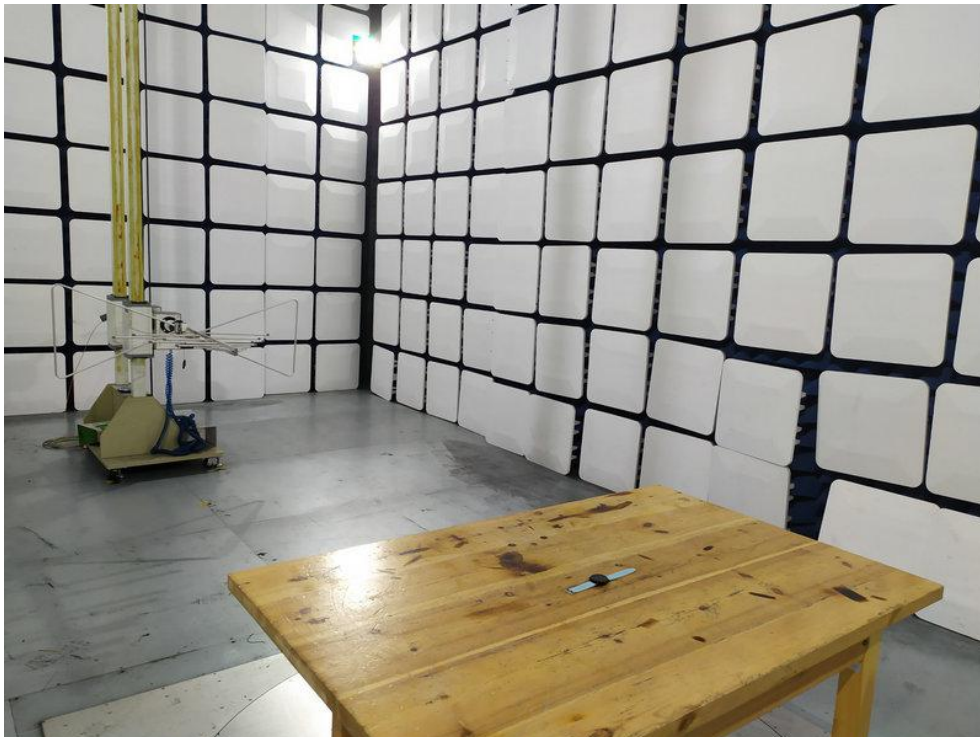
Photo of Radiation Emission Test
