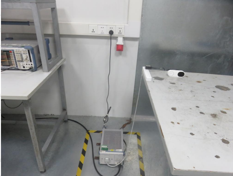
Photo of Power Line Conducted Emission Test
