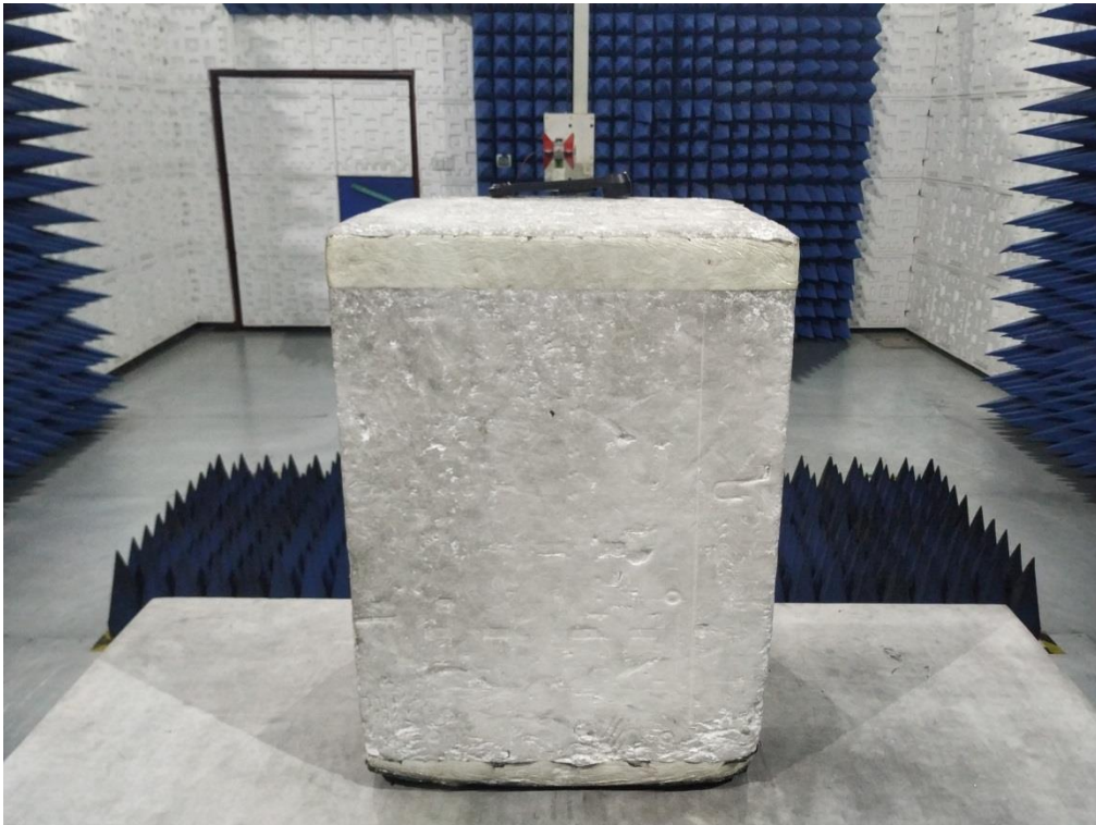
RADIATED EMISSION TEST SETUP ABOVE 1GHZ
