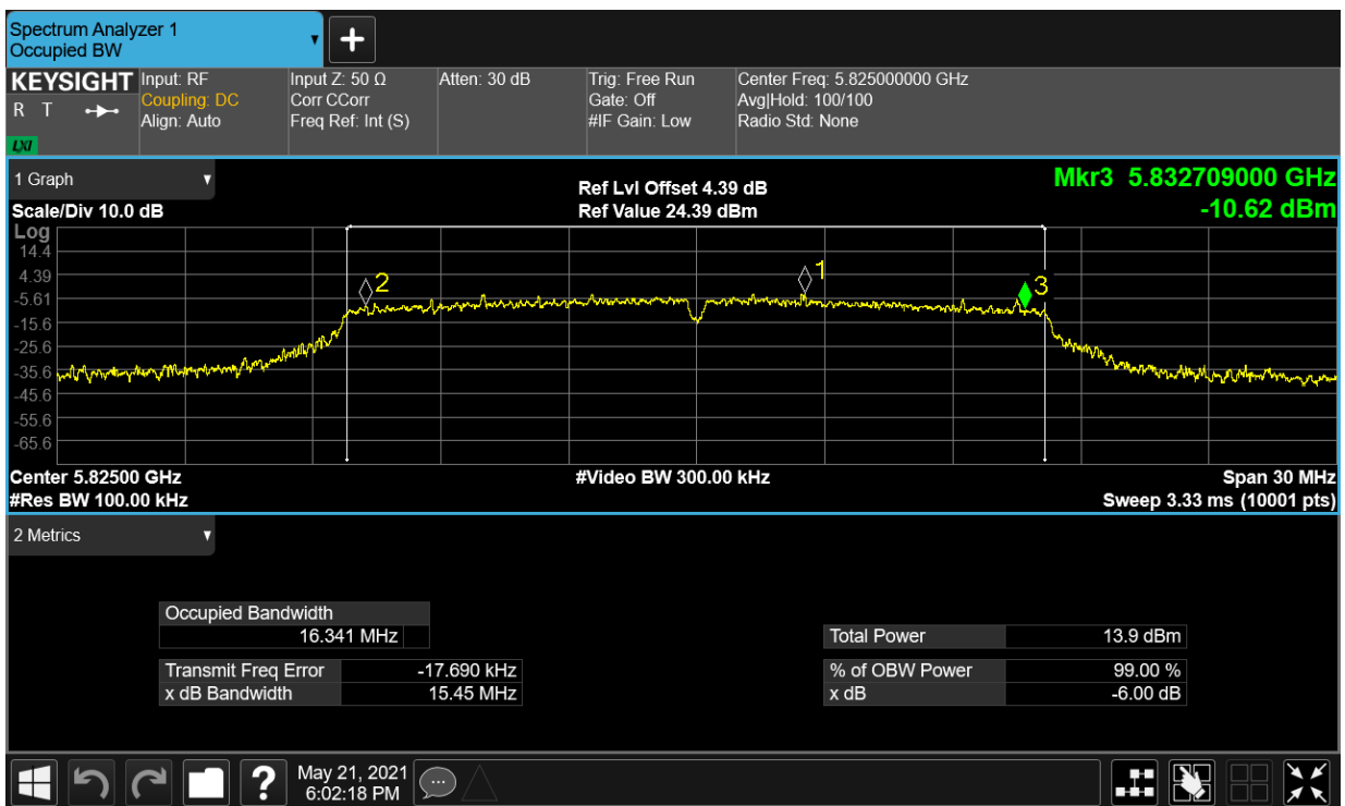
-6dB Bandwidth NVNT ac20 5745MHz Ant1
