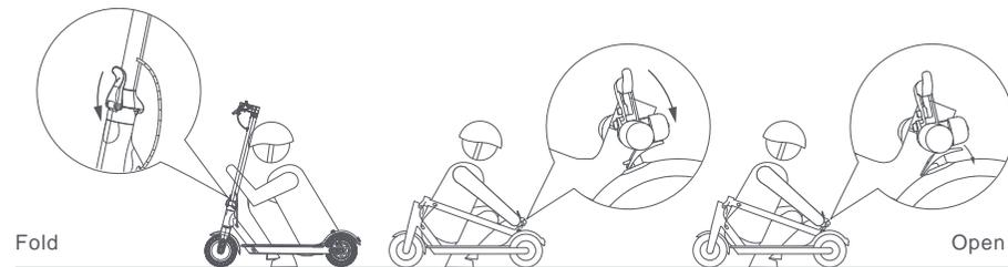
Make sure that the scooter's turned off. To fold, unlock the folding mechanism, and bend the handlebar stem to hook the buckle on the rear mudguard. To open, press the bell trigger to remove from the buckle, erect the handlebar and lock the folding structure.
