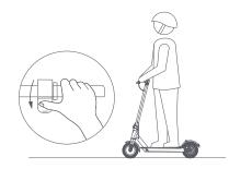
When the scooter starts to coast, put both feet on the deck and press the accelerator (the accelerator initiates once the coasting speed exceeds 3.1 mph)
