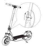
3. Tighten the screws onto both sides of the stem with the hexagon wrench
