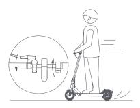
4 Release the accelerator and the kinetic energy recovery system (KERS) initiates automatically to brake slowly; And squeeze the brake lever for a sudden brake
