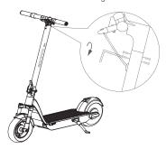
2. Attach the handlebar to the stem
