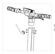
Put the handle bar set into the folding head tube, and keep the brake in the front.
