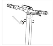
Keep the handle bar set in right position, then tighten the four M4\*14mm bolts with 4mm Allen wrench into the corresponding holes.
