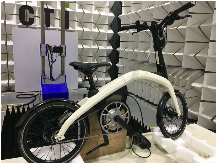
Radiated spurious emission Test Setup-2(Above 1GHz)
