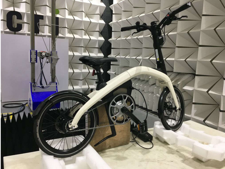
Radiated spurious emission Test Setup-1(Below 1GHz)
