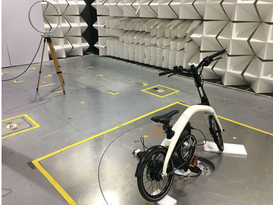
Radiated spurious emission Test Setup-1(Below 30MHz)
