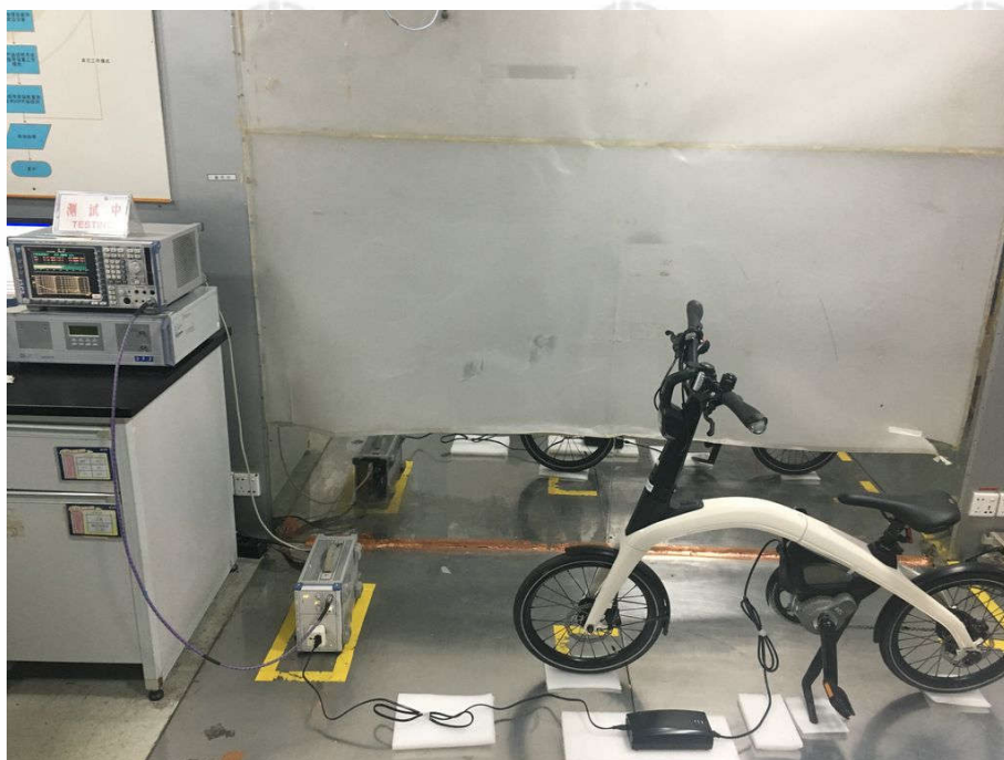
Conducted Emissions Test Setup
