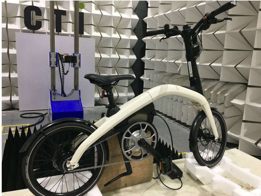
Radiated spurious emission Test Setup-3(Above 1GHz)
