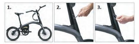
CAUTION: Ensure the steerer bolts are tight by standing with the front wheel between your legs. Twist the handlebar left and right to ensure it does not move.
