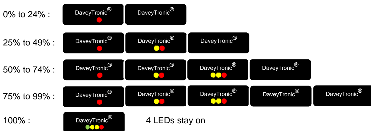
DBD LED sequence indicating battery level while charging
