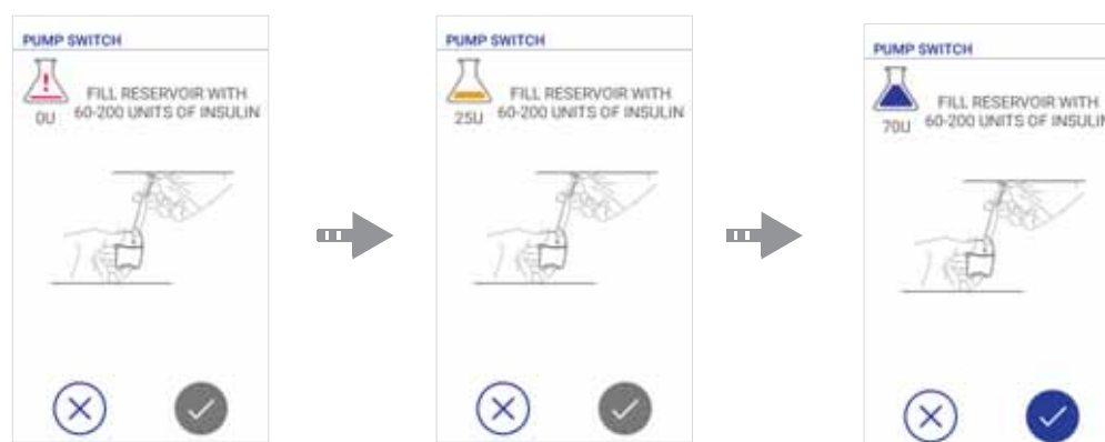
Figure 6-10 Filling Reservoir with Insulin
