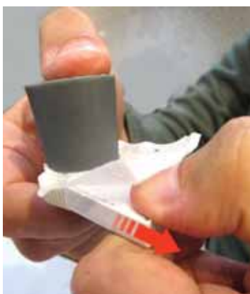
Figure 6-6 Separating Engine from Reservoir
