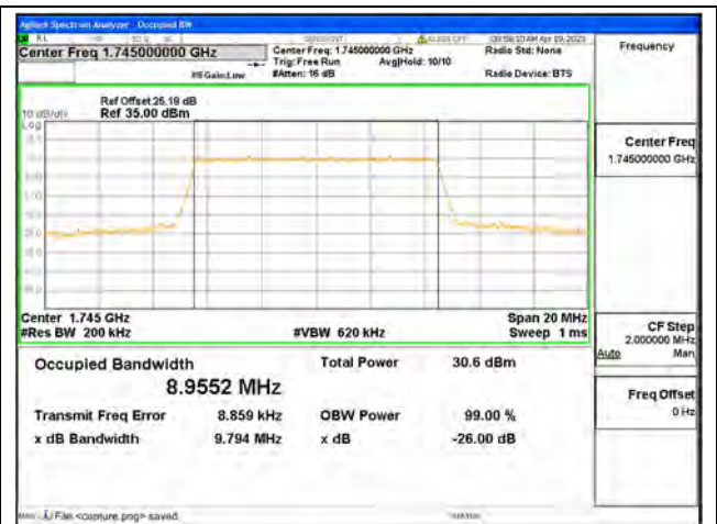
Band66 / 10MHz / 16QAM/ Mid CH
