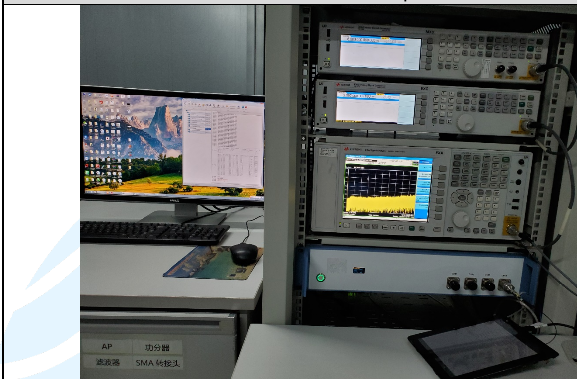
RF Conducted Test Setup
