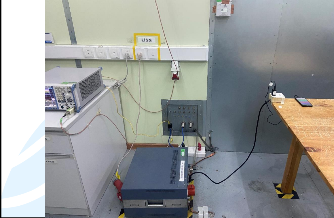
Conducted Emission Test Setup
