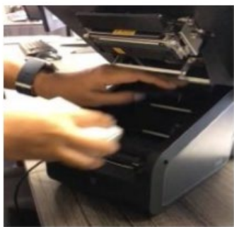
(3) Lift up on paper retainer to expose the paper bucket. (4) Insert thermal paper as shown. (5) Close lid.
