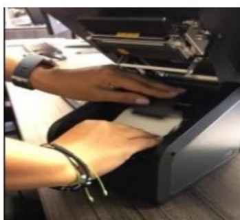
(3) Lift up on paper retainer to expose the paper bucket. (4) Insert thermal paper as shown. (5) Close lid.
