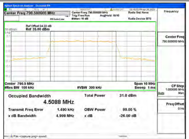
Band14 / 5MHz / 16QAM/ Low CH
