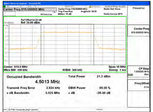
Band18 part90 / 5MHz / QPSK/ Mid CH
