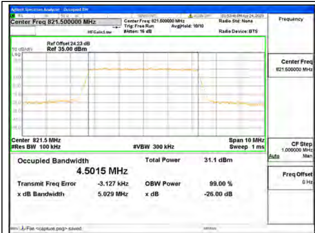
Band18 part90 / 5MHz / QPSK/ High CH
