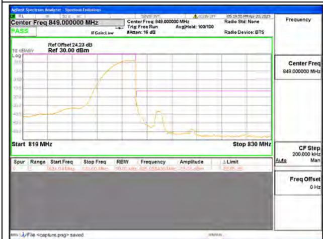
Band26 Part90 / 3MHz / High CH / QPSK / 1 RB
