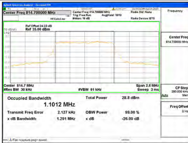
Band26 Part90 / 1.4MHz / 64QAM/ Low CH
