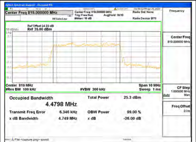
Band26 Part90 / 5MHz / 64QAM/ Mid CH
