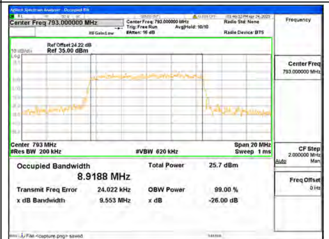
Band14 / 10MHz / 64QAM/ Mid CH
