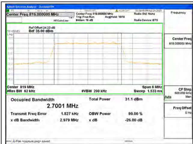
Band26 Part90 / 3MHz / QPSK/ Mid CH
