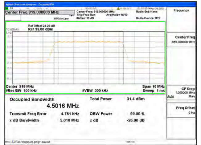
Band26 Part90 / 5MHz / QPSK/ Mid CH
