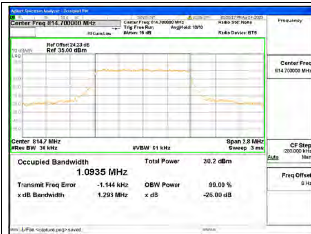
Band26 Part90 / 1.4MHz / QPSK/ Low CH
