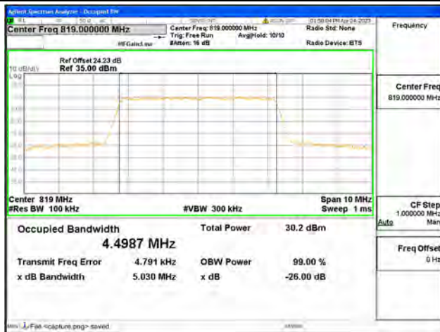
Band26 Part90 / 5MHz / 16QAM/ Mid CH
