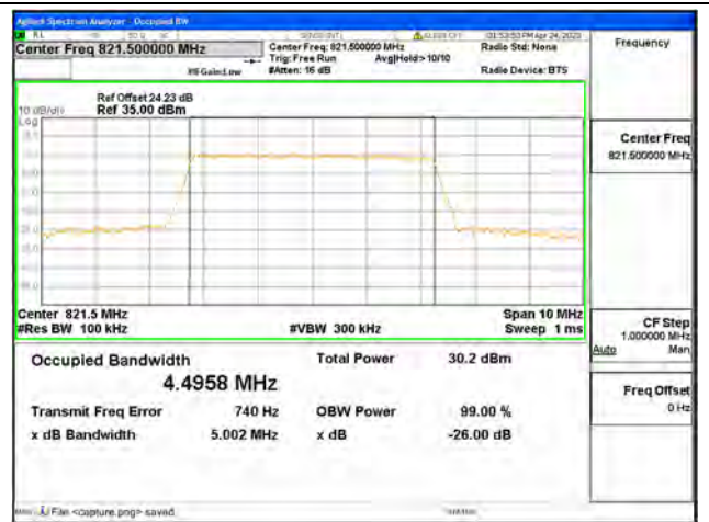
Band18 part90 / 5MHz / 16QAM/ High CH
