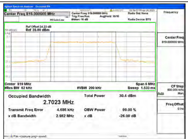
Band26 Part90 / 3MHz / 16QAM/ Mid CH
