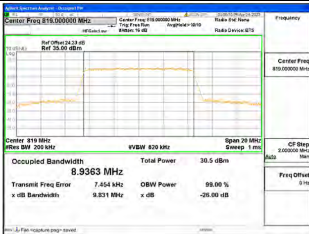
Band26 Part90 / 10MHz / 16QAM/ Mid CH
