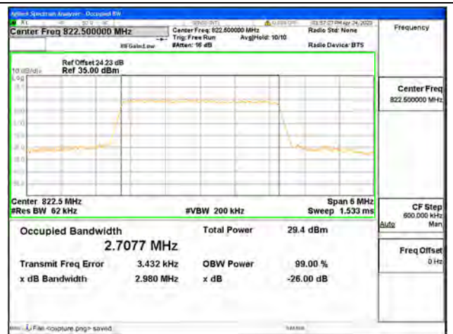
Band26 Part90 / 3MHz / 64QAM/ High CH
