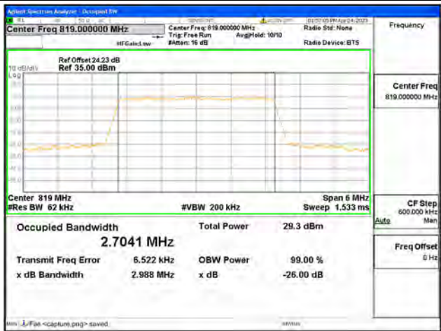
Band26 Part90 / 3MHz / 64QAM/ Mid CH
