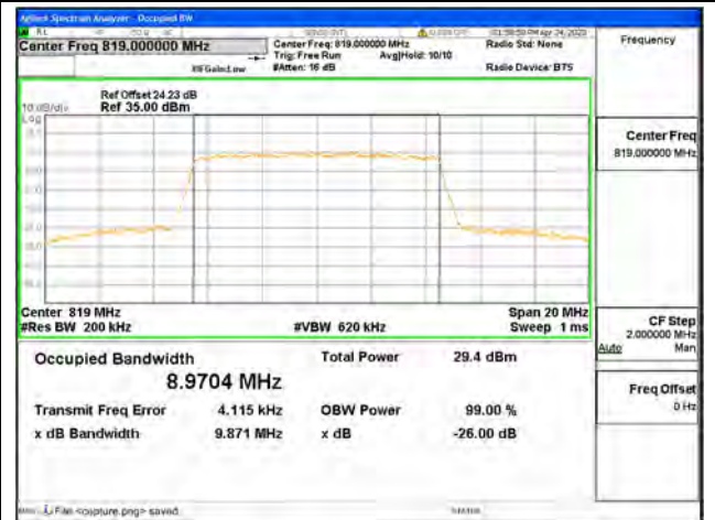
Band26 Part90 / 10MHz / 64QAM/ Mid CH
