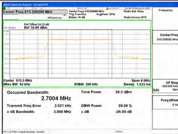
Band26 Part90 / 3MHz / 16QAM/ Low CH
