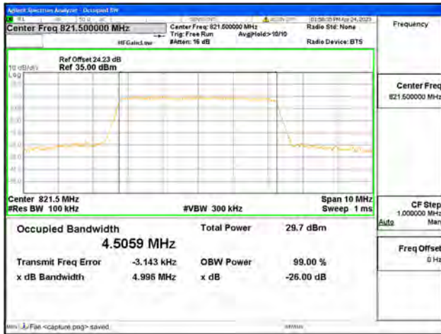
Band26 Part90 / 5MHz / 64QAM/ High CH
