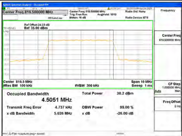
Band18 part90 / 5MHz / 16QAM/ Mid CH
