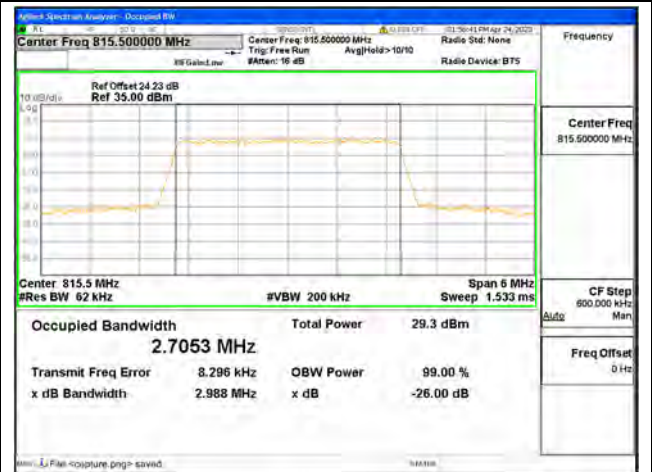
Band26 Part90 / 3MHz / 64QAM/ Low CH
