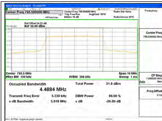
Band14 / 5MHz / QPSK/ High CH
