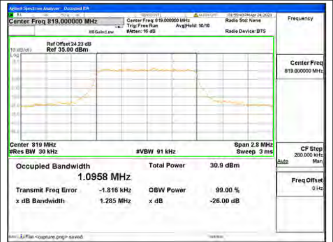
Band26 Part90 / 1.4MHz / QPSK/ Mid CH
