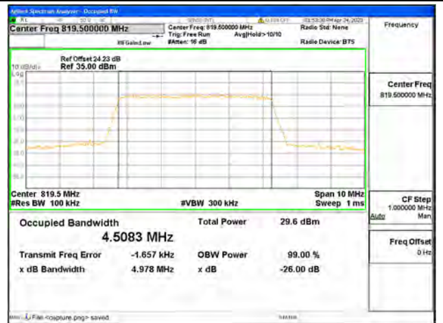
Band18 part90 / 5MHz / 64QAM/ Mid CH
