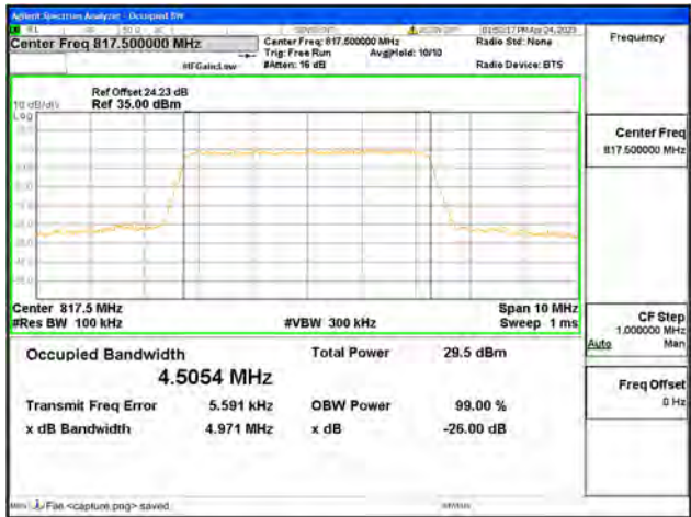
Band18 part90 / 5MHz / 64QAM/ Low CH
