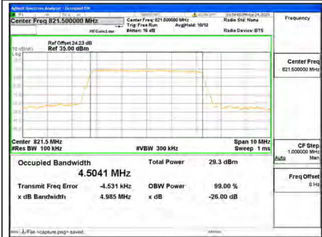
Band18 part90 / 5MHz / 64QAM/ High CH
