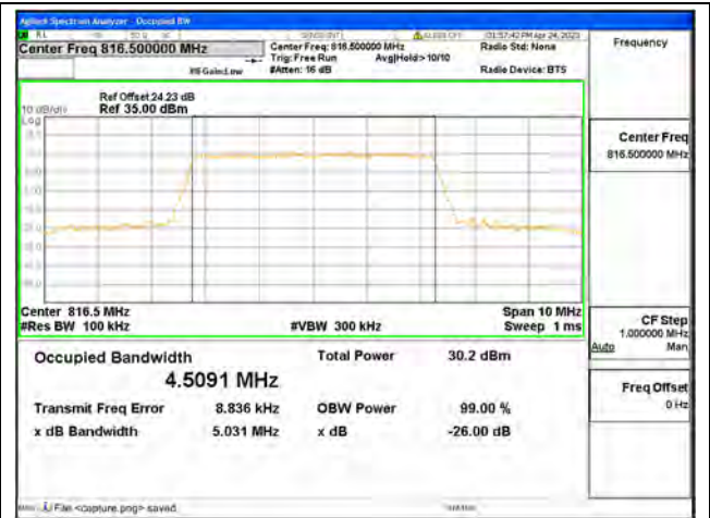
Band26 Part90 / 5MHz / 16QAM/ Low CH
