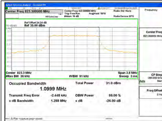
Band26 Part90 / 1.4MHz / QPSK/ High CH
