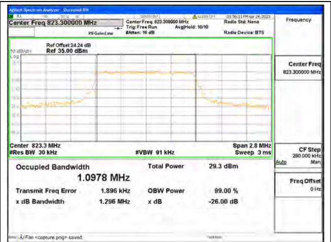
Band26 Part90 / 1.4MHz / 16QAM/ High CH
