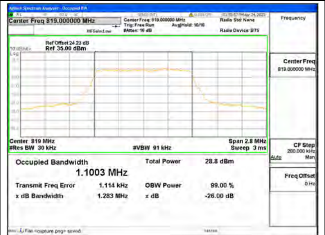
Band26 Part90 / 1.4MHz / 64QAM/ Mid CH
