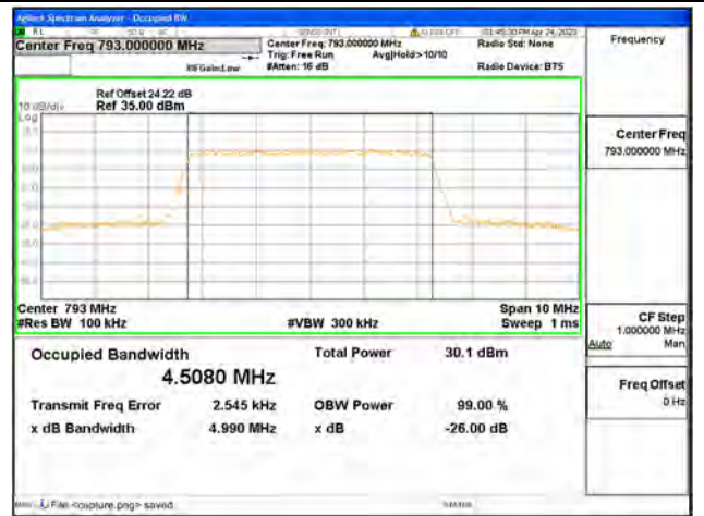
Band14 / 5MHz / 64QAM/ Mid CH
