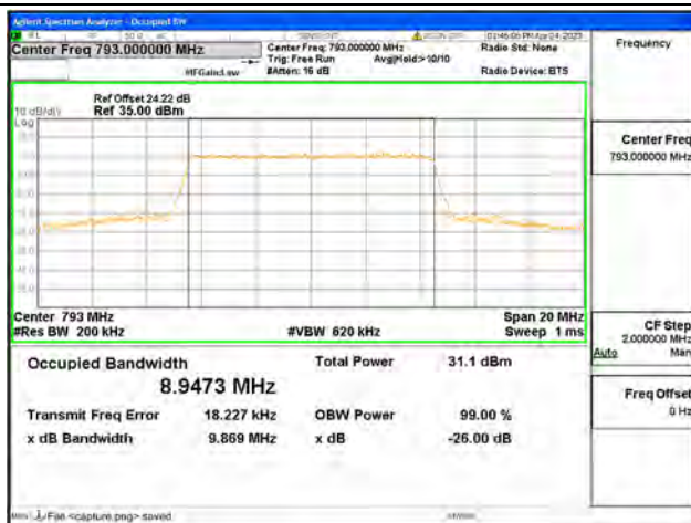
Band14 / 10MHz / 16QAM/ Mid CH
