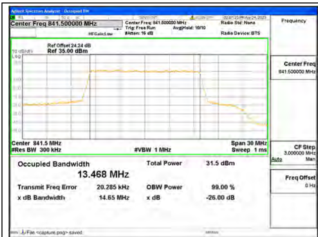
Band26 Part22 / 15MHz / QPSK/ High CH
