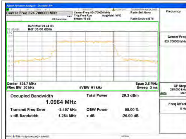
Band26 Part22 / 1.4MHz / QPSK/ Low CH
