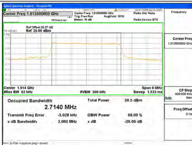
Band25 / 3MHz / 16QAM/ High CH
