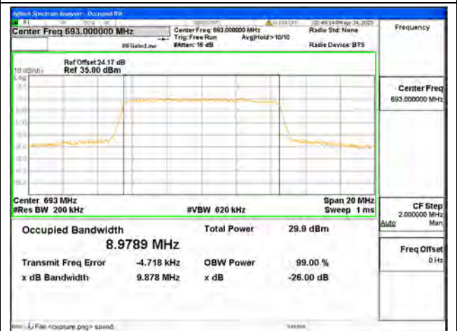
Band71 / 10MHz / 64QAM/ High CH
