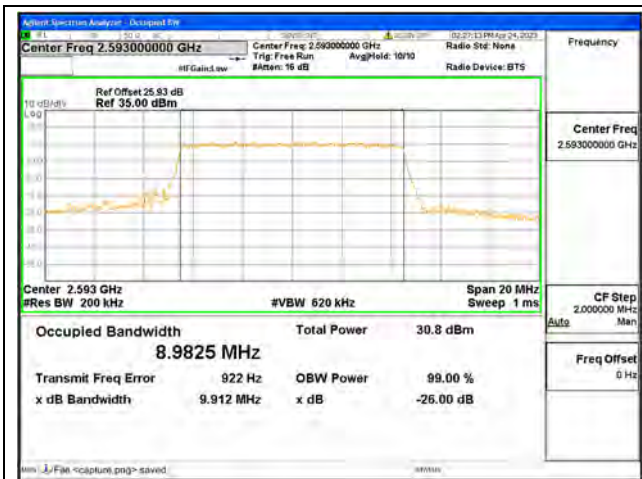
Band41 / 10MHz / QPSK/ Mid CH
