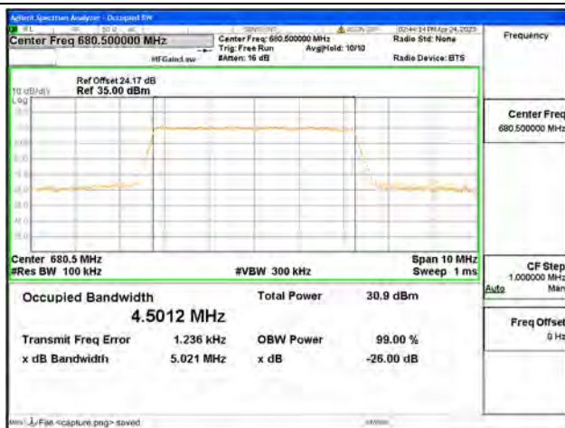
Band71 / 5MHz / 16QAM/ Mid CH
