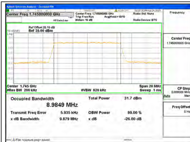
Band66 / 10MHz / QPSK/ Mid CH
