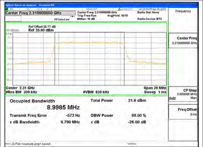
Band30 / 10MHz / QPSK/ Mid CH
