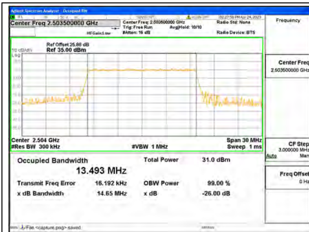
Band41 / 15MHz / QPSK/ Low CH
