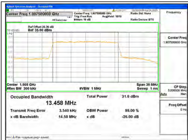
Band25 / 15MHz / QPSK/ High CH
