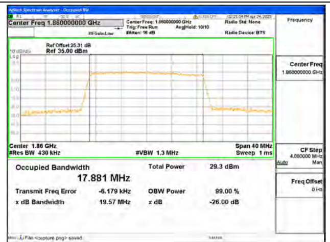
Band25 / 20MHz / 64QAM/ Low CH
