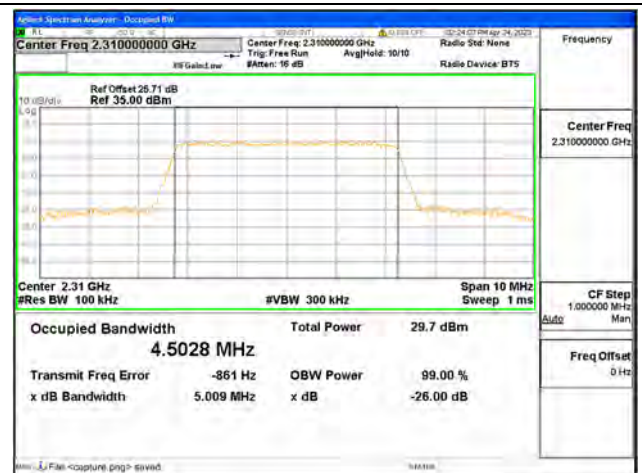
Band30 / 5MHz / 64QAM/ Mid CH
