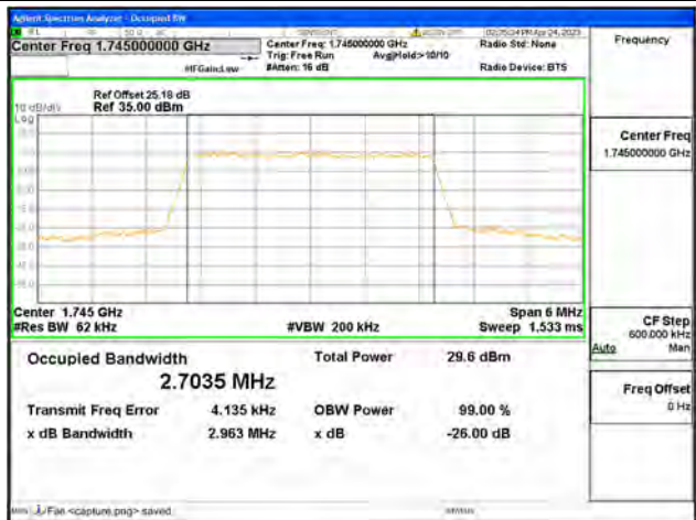
Band66 / 3MHz / 64QAM/ Mid CH
