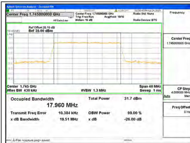
Band66 / 20MHz / QPSK/ Mid CH
