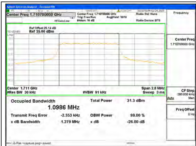
Band66 / 1.4MHz / QPSK/ Low CH
