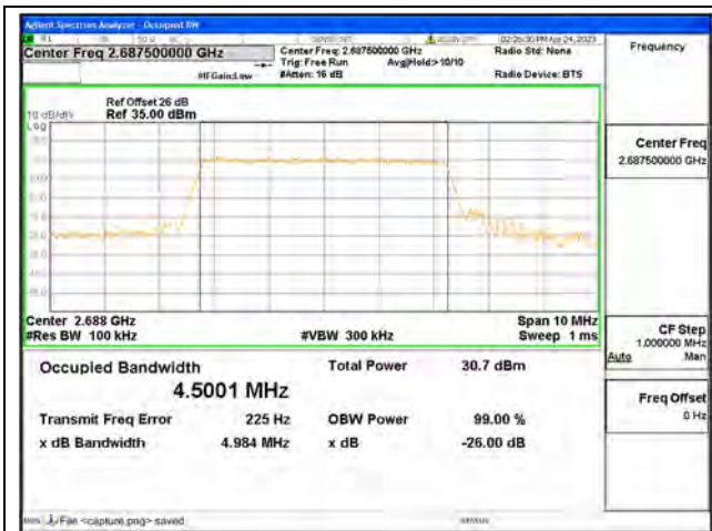
Band41 / 5MHz / QPSK/ High CH
