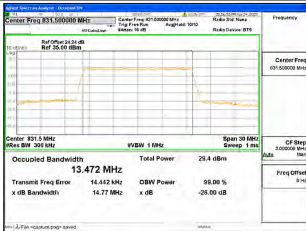
Band26 Part22 / 15MHz / 64QAM/ Low CH
