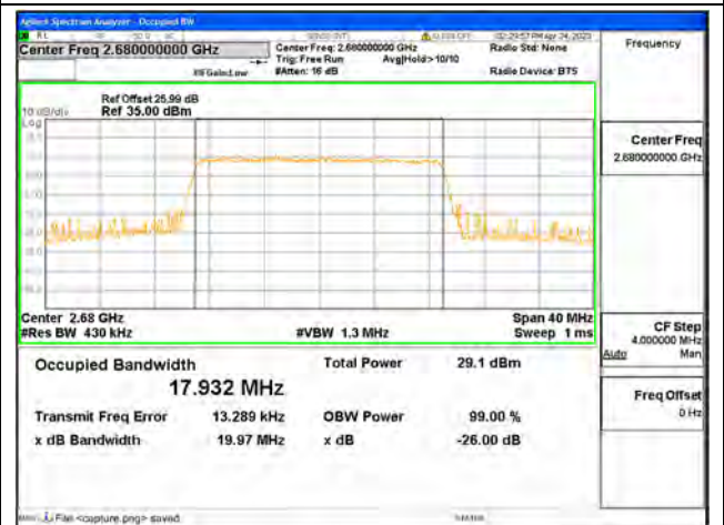
Band41 / 20MHz / 64QAM/ High CH
