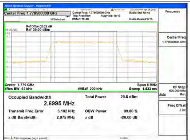
Band66 / 3MHz / 64QAM/ High CH
