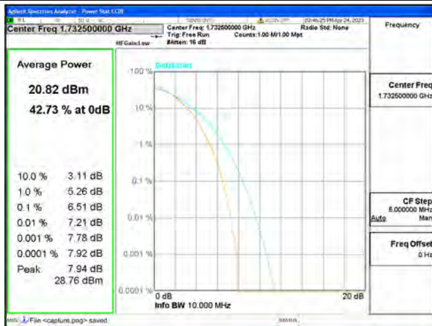
Band4 / 10MHz / Mid CH / 64QAM
