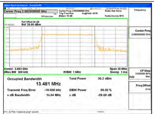
Band41 / 15MHz / 16QAM/ High CH
