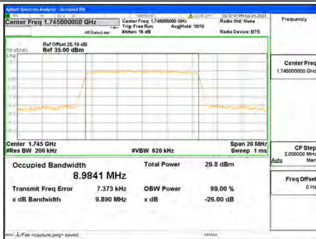
Band66 / 10MHz / 64QAM/ Mid CH
