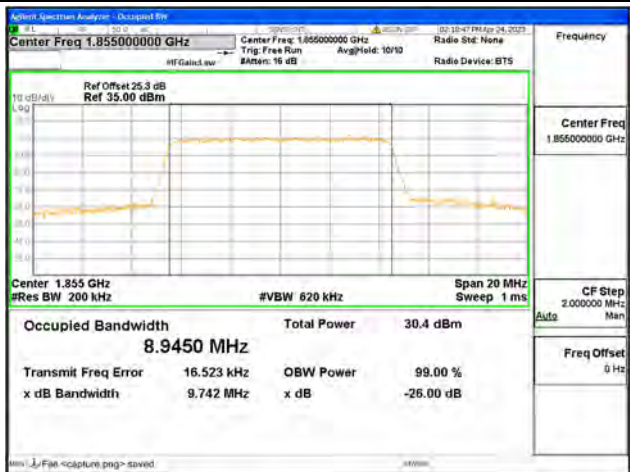
Band25 / 10MHz / 16QAM/ Low CH
