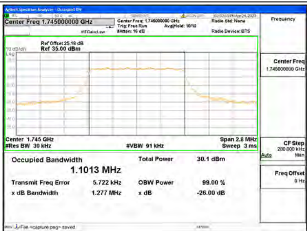
Band66 / 1.4MHz / 16QAM/ Mid CH
