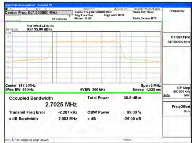
Band26 Part22 / 3MHz / QPSK/ High CH
