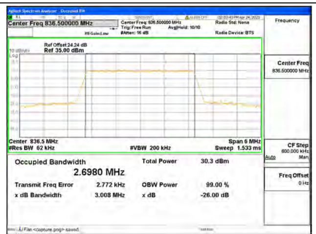
Band26 Part22 / 3MHz / 16QAM/ Mid CH
