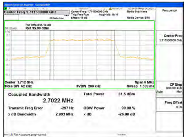
Band66 / 3MHz / QPSK/ Low CH
