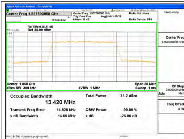
Band25 / 15MHz / QPSK/ Low CH
