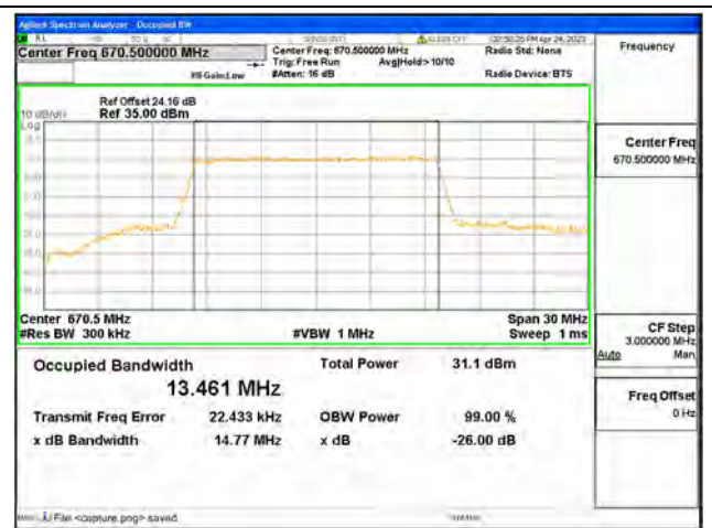
Band71 / 15MHz / 16QAM/ Low CH
