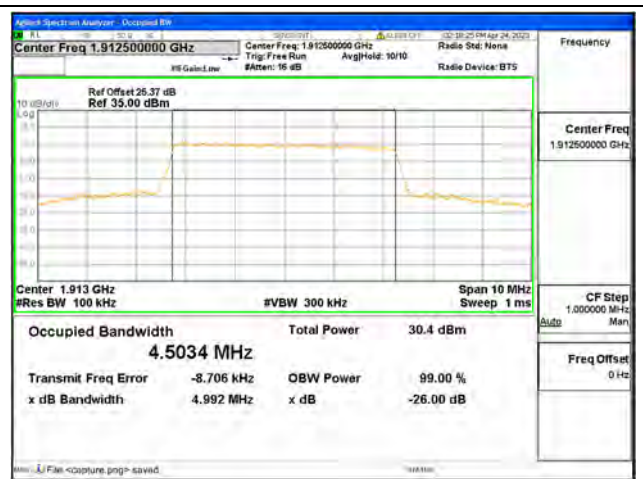
Band25 / 5MHz / 16QAM/ High CH
