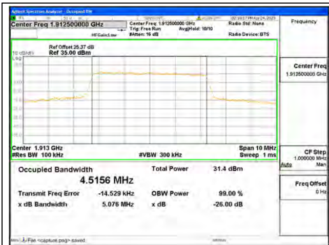
Band25 / 5MHz / QPSK/ High CH
