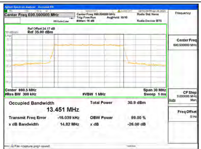
Band71 / 15MHz / 16QAM/ High CH
