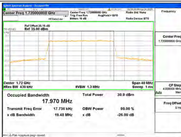
Band66 / 20MHz / 16QAM/ Low CH
