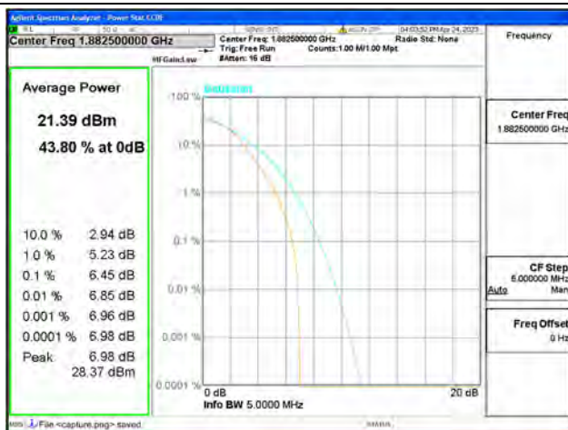
Band25 / 1.4MHz / Mid CH / 16QAM
