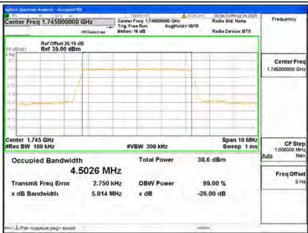
Band66 / 5MHz / 16QAM/ Mid CH
