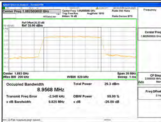
Band25 / 10MHz / 64QAM/ Mid CH
