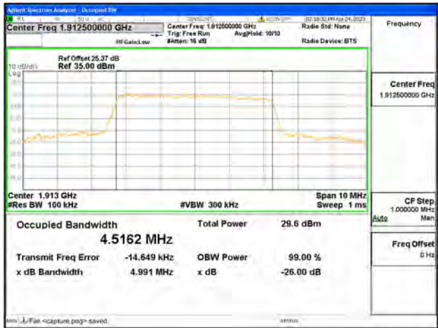
Band25 / 5MHz / 64QAM/ High CH
