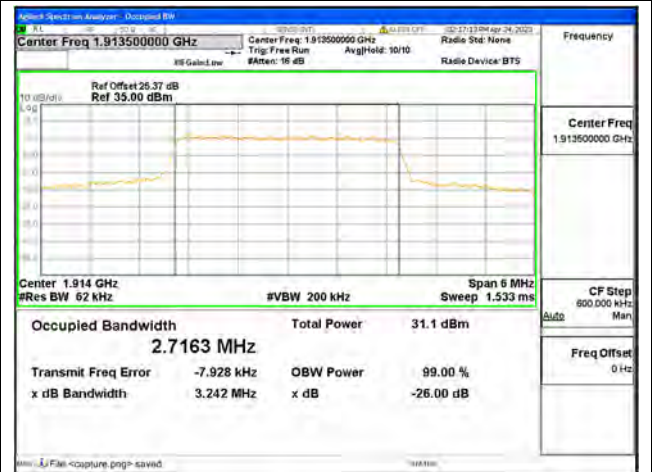
Band25 / 3MHz / QPSK/ High CH
