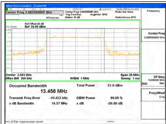
Band41 / 15MHz / QPSK/ High CH
