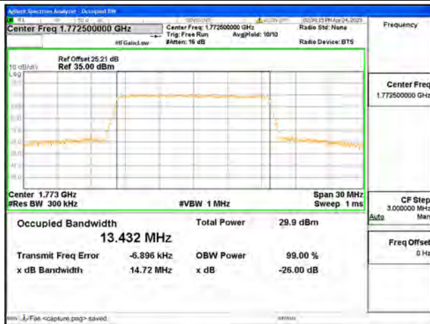
Band66 / 15MHz / 64QAM/ High CH
