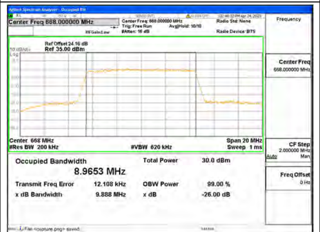
Band71 / 10MHz / 64QAM/ Low CH
