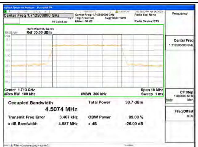
Band66 / 5MHz / 16QAM/ Low CH
