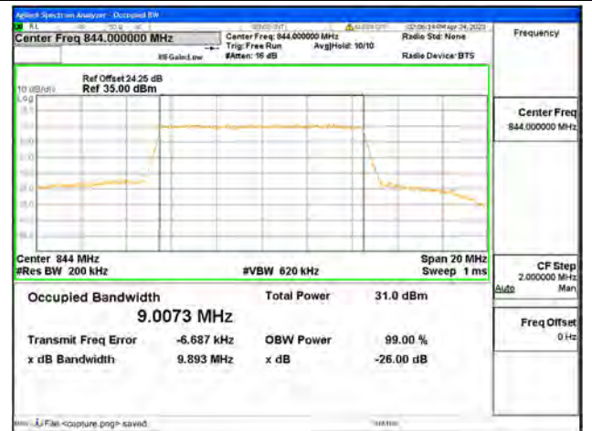
Band26 Part22 / 10MHz / QPSK/ High CH
