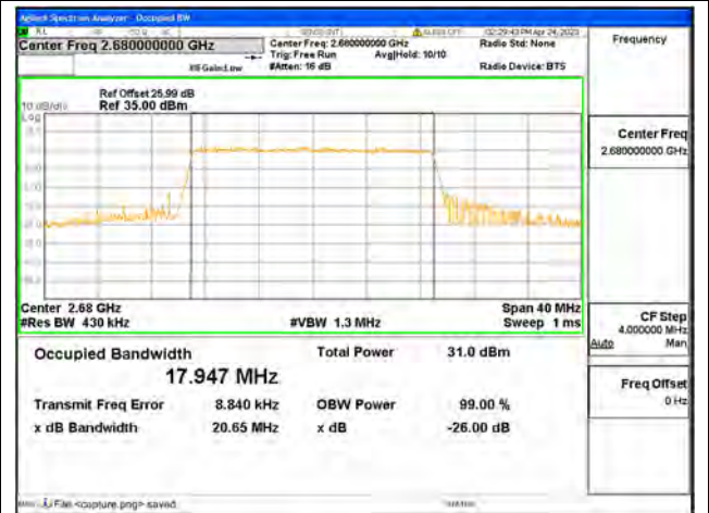
Band41 / 20MHz / QPSK/ High CH
