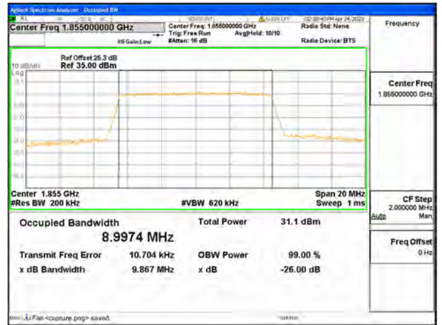
Band25 / 10MHz / QPSK/ Low CH
