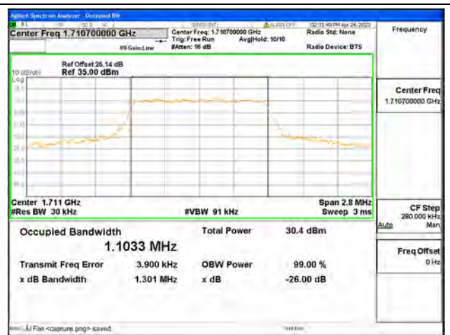
Band66 / 1.4MHz / 16QAM/ Low CH
