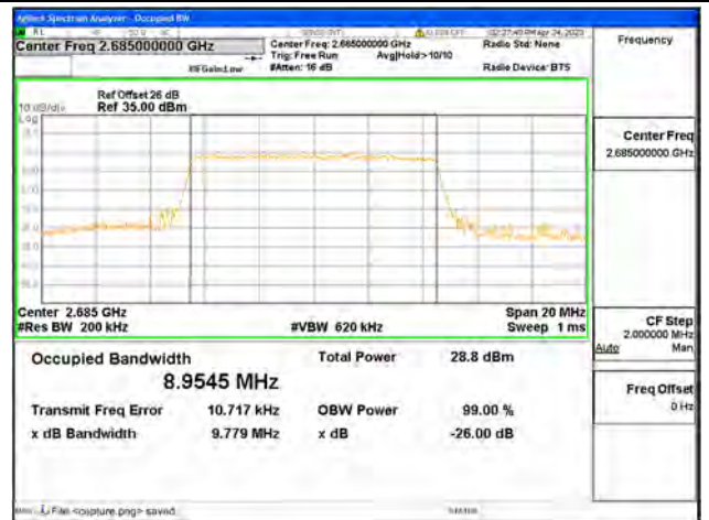
Band41 / 10MHz / 64QAM/ High CH
