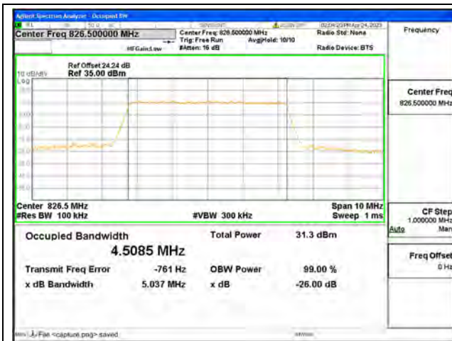
Band26 Part22 / 5MHz / QPSK/ Low CH
