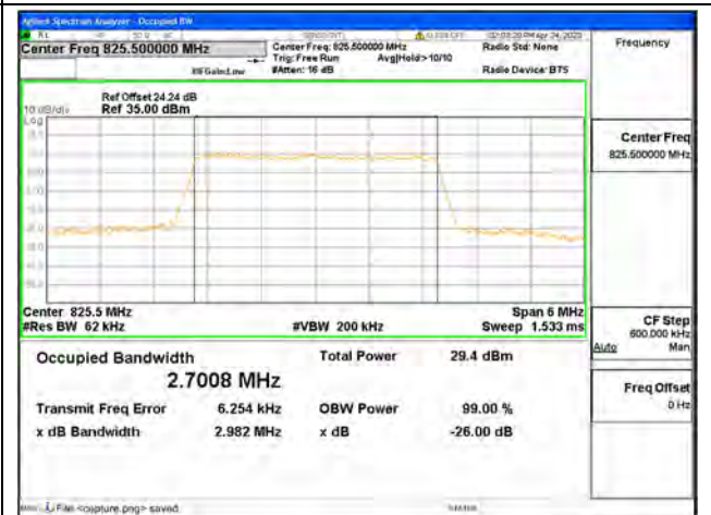
Band26 Part22 / 3MHz / 64QAM/ Low CH
