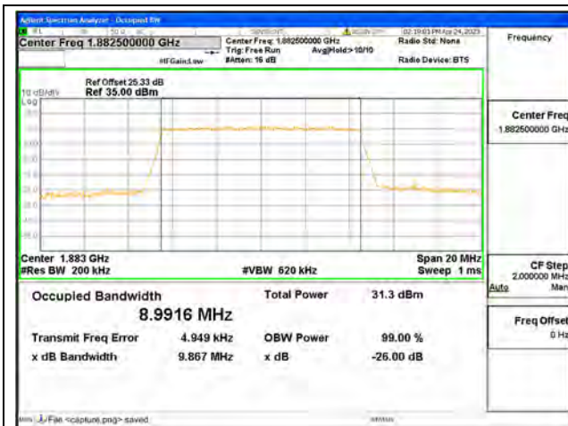
Band25 / 10MHz / QPSK/ Mid CH
