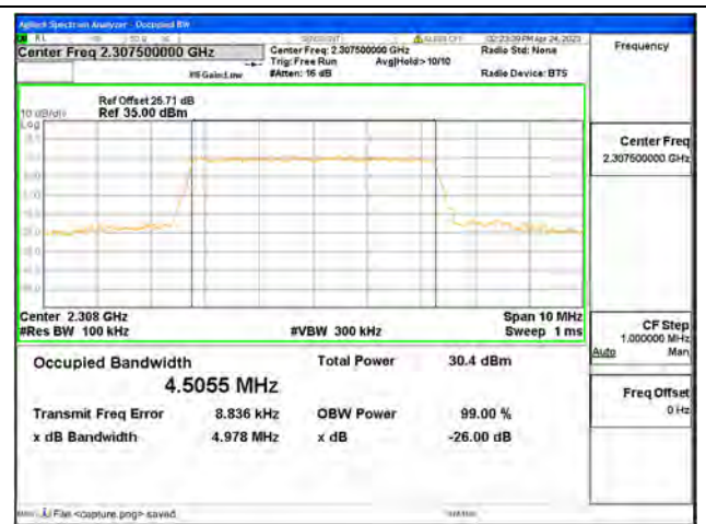
Band30 / 5MHz / 16QAM/ Low CH
