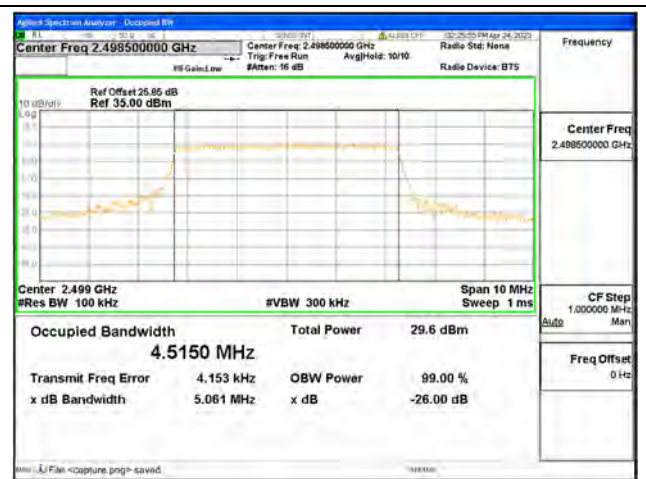
Band41 / 5MHz / 16QAM/ Low CH
