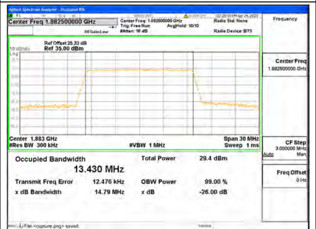
Band25 / 15MHz / 64QAM/ Mid CH
