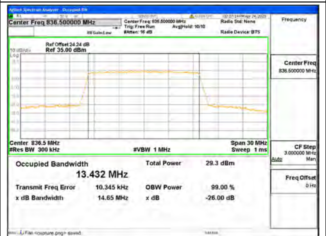
Band26 Part22 / 15MHz / 64QAM/ Mid CH
