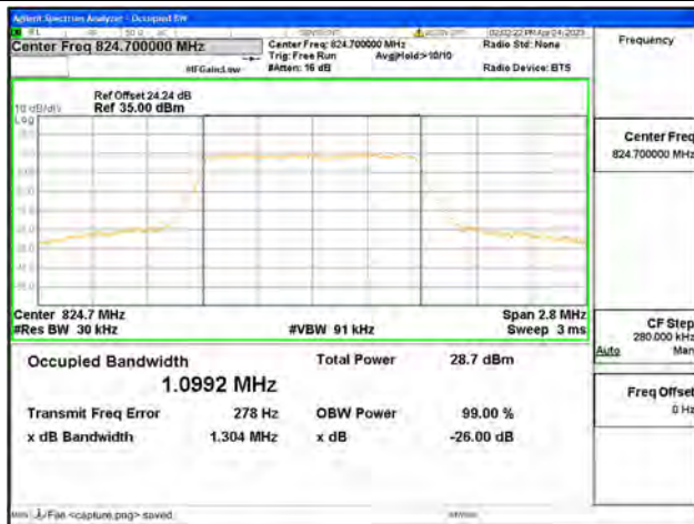
Band26 Part22 / 1.4MHz / 64QAM/ Low CH
