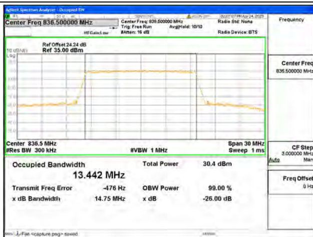
Band26 Part22 / 15MHz / 16QAM/ Mid CH
