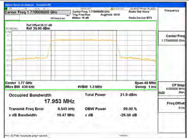
Band66 / 20MHz / QPSK/ High CH
