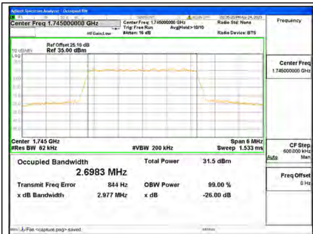
Band66 / 3MHz / QPSK/ Mid CH
