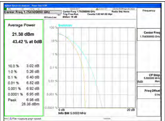
Band4 / 1.4MHz / High CH / 16QAM
