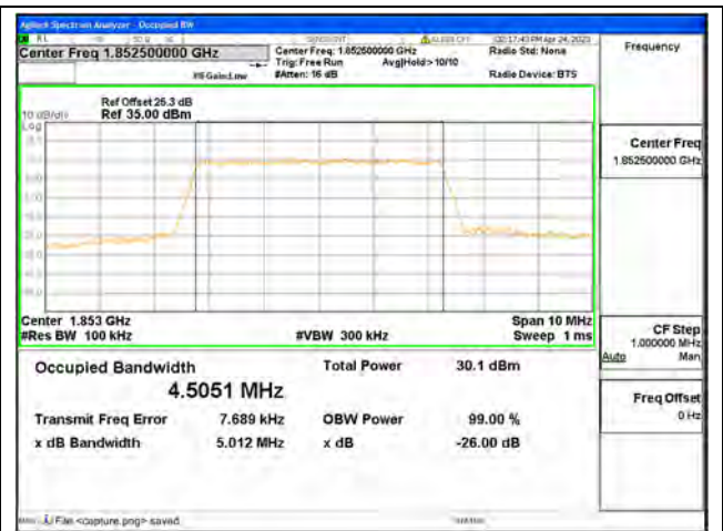
Band25 / 5MHz / 16QAM/ Low CH
