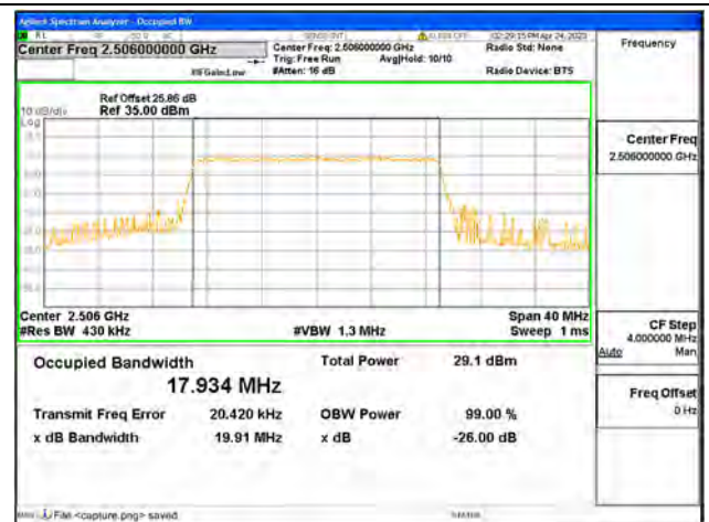
Band41 / 20MHz / 64QAM/ Low CH
