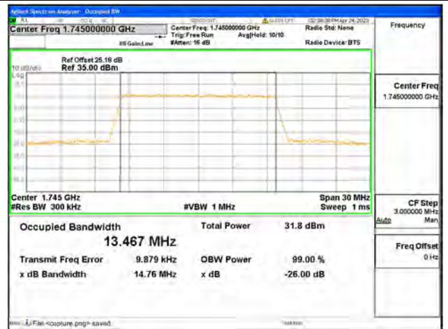
Band66 / 15MHz / QPSK/ Mid CH
