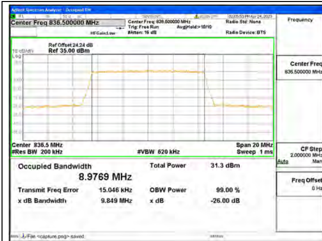
Band26 Part22 / 10MHz / QPSK/ Mid CH
