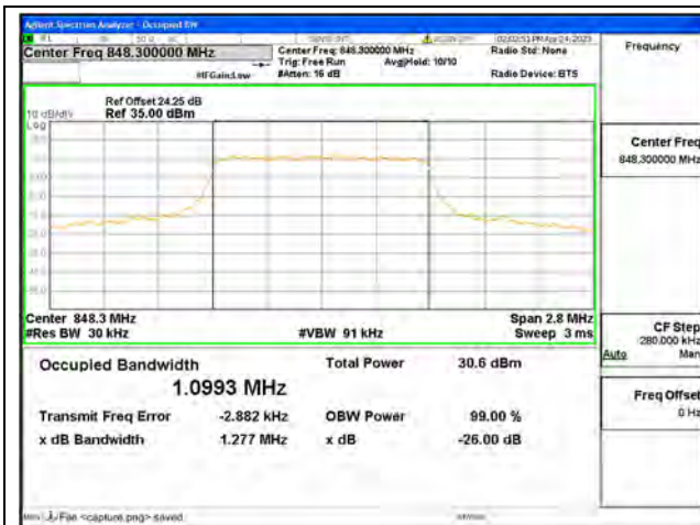
Band26 Part22 / 1.4MHz / QPSK/ High CH
