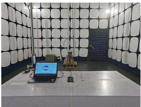
3. Radiated emission (9KHz-30MHz)
