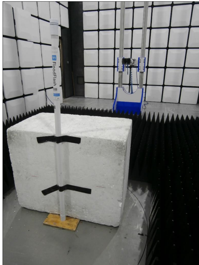
Figure 5 - Test Setup - 1 GHz to 5 GHz
