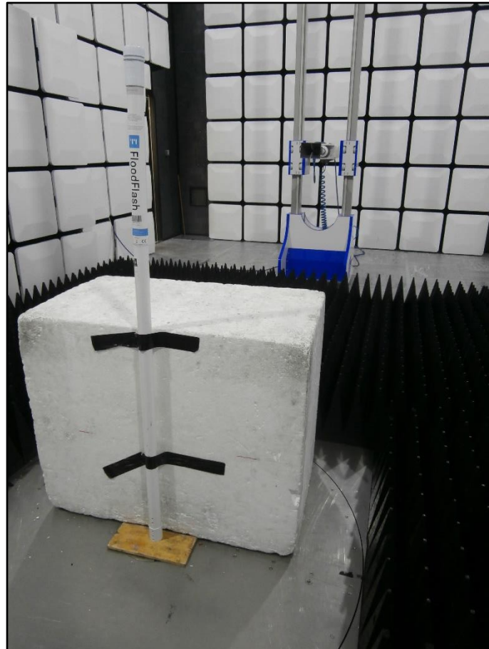
Figure 7 - Test Setup - 1 GHz to 10 GHz
