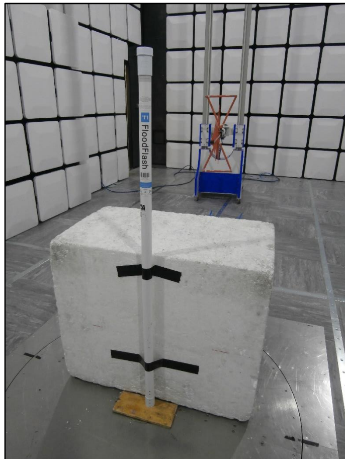
Figure 6 - Test Setup - 30 MHz to 1 GHz
