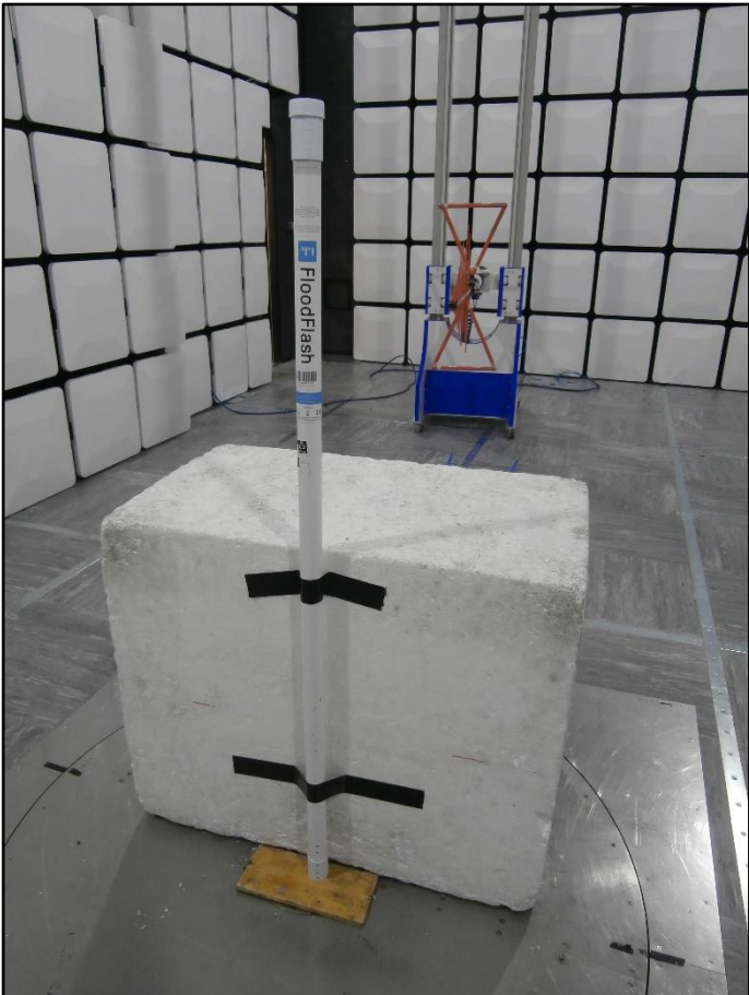
Figure 4 - Test Setup - 30 MHz to 1 GHz
